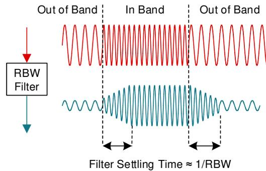
**Figure 3. Settling Time Effects of the RBW Filter**
