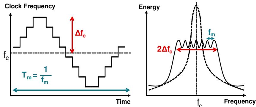
**Figure 2. Triangular Modulation in the Time (Left) and Frequency Domain (Right)**
