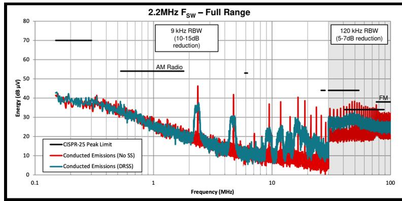
Figure 6. Conduction EMI Reduction by DRSS (LM5156, Switching at 2.2 MHz)
