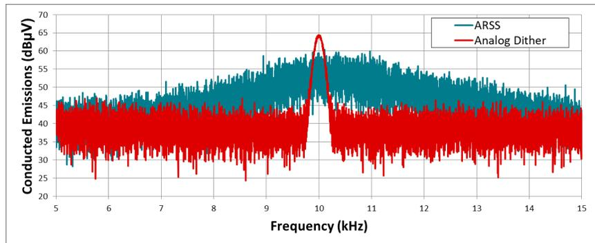
Figure 4. ARSS Improves Audible Noise by Spreading the 10-kHz Tone
