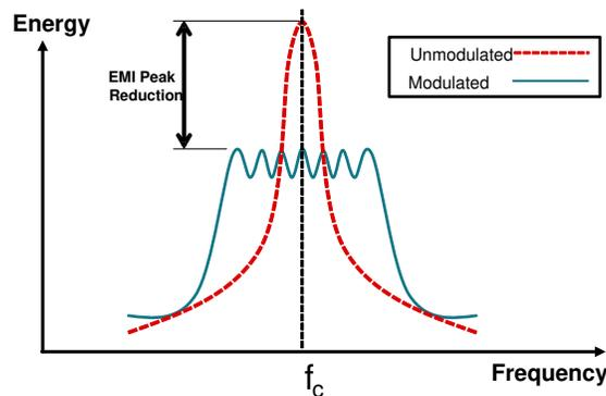
**Figure 1. EMI Reduction by Spread Spectrum, Frequency Modulation**
