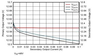
Figure 5-12. Load Regulation vs Secondary Output Current
