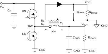
Figure 2-1. General Fly-Buck Converter Circuit
