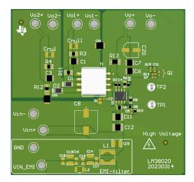
Figure 5-2. LMR38020 Fly-Buck Demo Board
