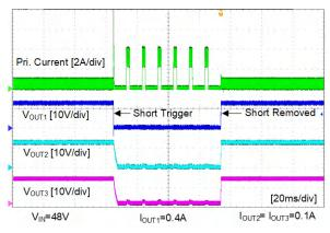
Figure 5-13. Short Circuit On Primary Output
