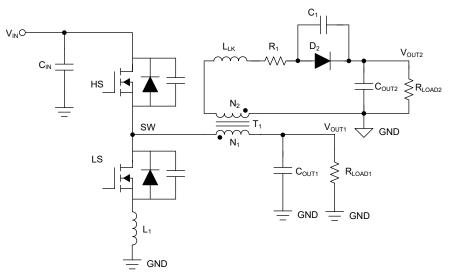
Figure 3-2. Fly-Buck Converter Circuit Considering Parasitic
