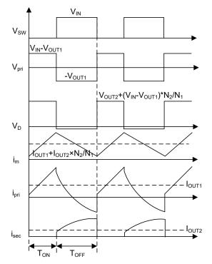
Figure 3-1. Fly-Buck<sup>™</sup> Steady State Operation Waveforms
