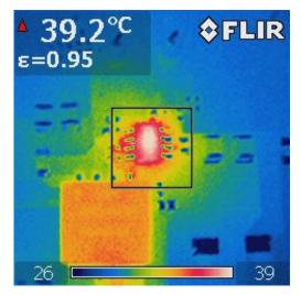
Figure 5-15. Thermal Performance When V<sub>IN</sub>=48 V, Full Load
