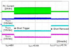
Figure 5-14. Short Circuit On Secondary Output
