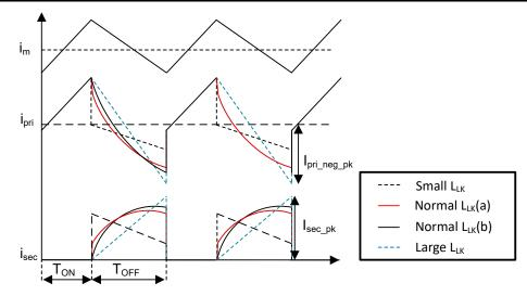
Figure 3-3. Current Waveforms Affected by Leakage Inductance
