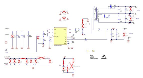
Figure 5-1. LMR38020 Fly-Buck Converter Schematic
