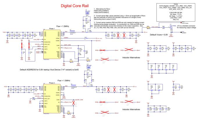
Figure 3-4. TPS6287B25 Schematic for Digital Core Rail
