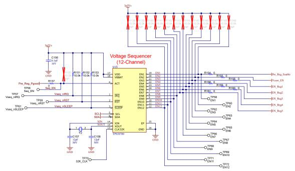
Figure 12-1. 12-Channel Sequencer Sub-Circuit Schematic
