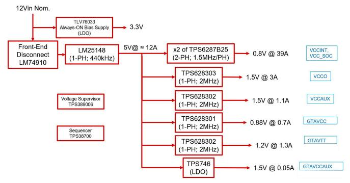
Figure 2-1. VE2302 Device Minimum Rails Configuration Power Tree Block Diagram
