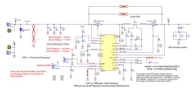
Figure 3-1. LM74910 Schematic for Front-End Protection
