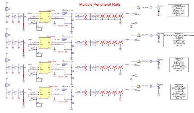
Figure 3-5. TPS62830x Schematics for Multiple Peripheral Rails
