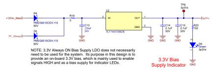
Figure 3-2. TLV76033 Schematic for 3.3V Always-ON Bias Supply
