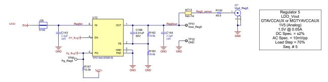
Figure 3-6. TPS746 Schematic for GTAVCCAUX Rail
