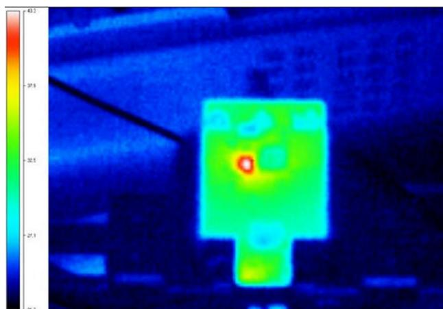
Figure 1. LM27402 Thermal Performance
