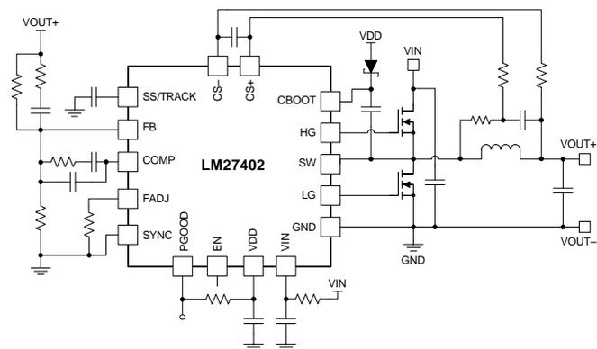
Figure 4. LM27402 Synchronous Buck Controller
