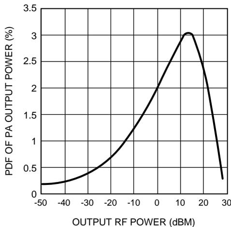
**Figure 4. Probability of PA Output Level in a 3G CDMA Mobile Unit**
