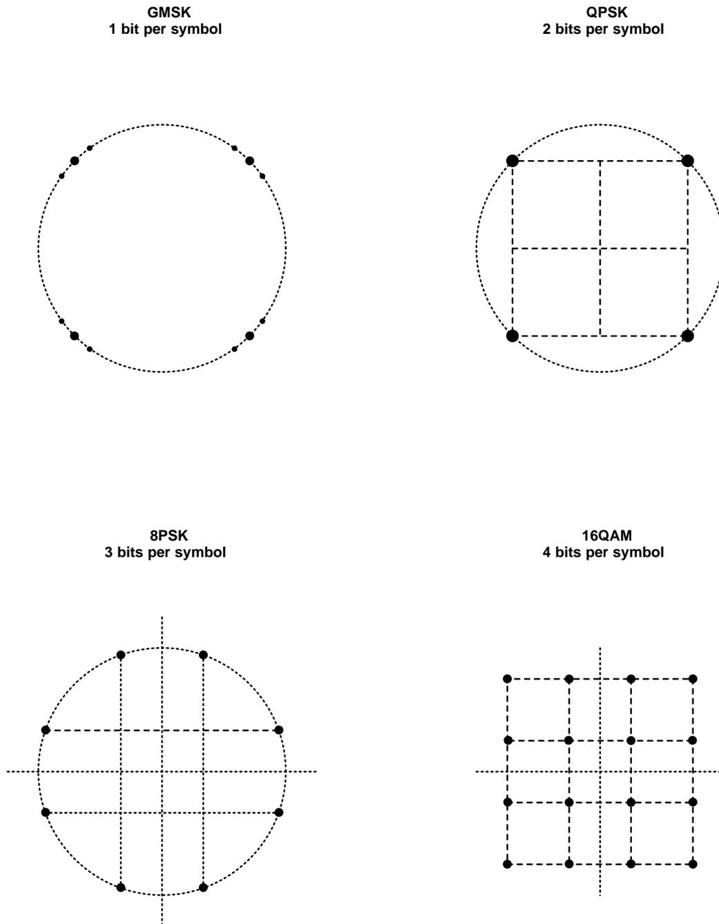
**Figure 1. Constellation Diagram of Digital Modulation Used in Cellular Phones**
