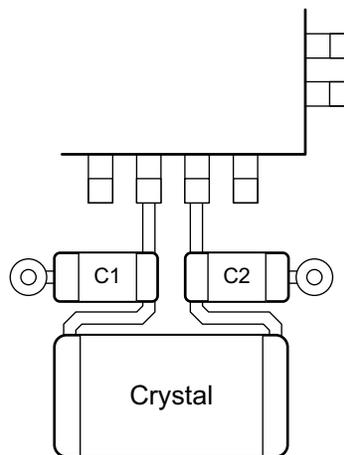
Figure 3. Recommended Layout for Small Surface-Mount Crystal
