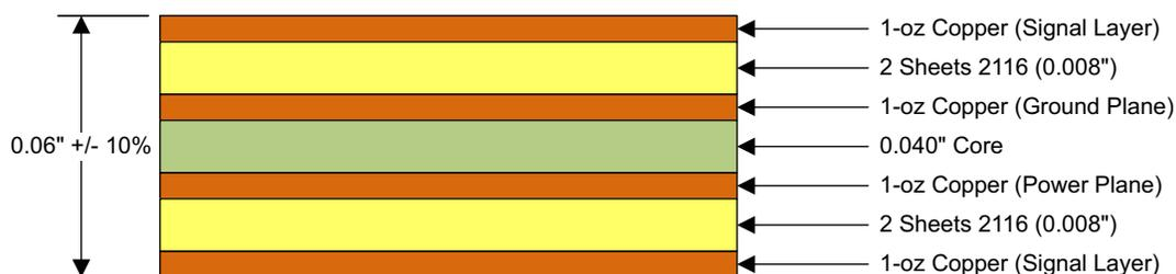
**Figure 5. Typical Four-Layer PCB Stack with Routing Assignments**
