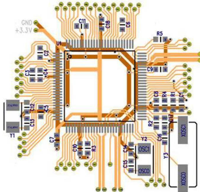
**Figure 13. Stellaris LM3S9B90 Microcontroller Minimal Circuit**
