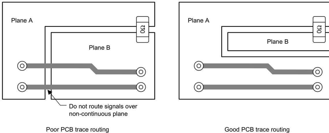
**Figure 11. Examples of PCB Trace Layout**
