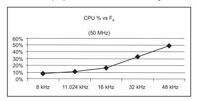
Figure 7. CPU Utilization Graph Based on Audio Sampling Frequency
