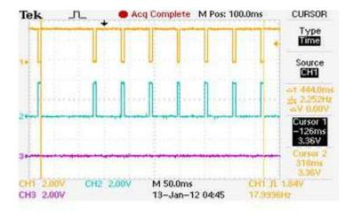
Figure 6. 8-kHz Interrupt Waveforms
