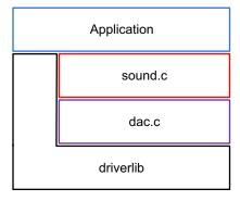
Figure 4. Dual-SPI Application Software Stack
