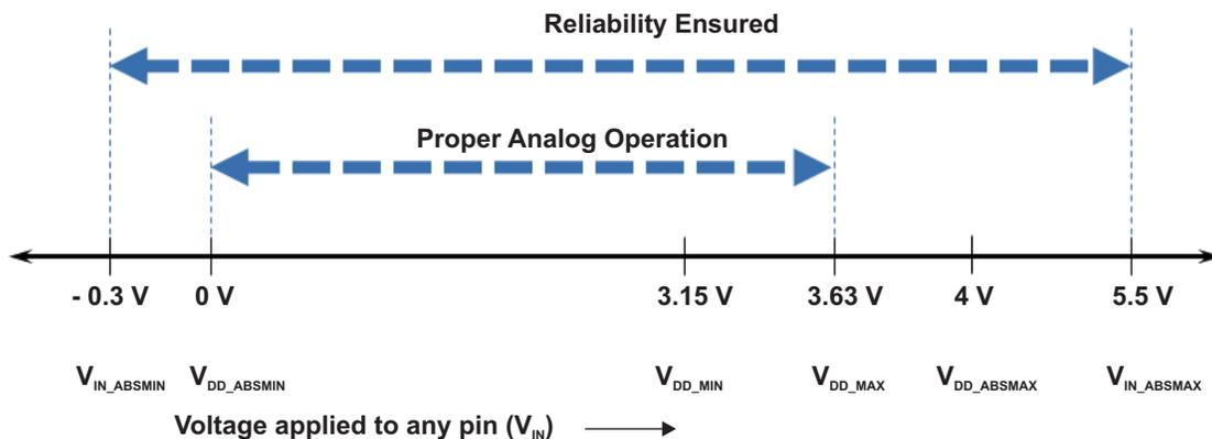
**Figure 2. Regions of Reliability and Proper Analog Operation**
