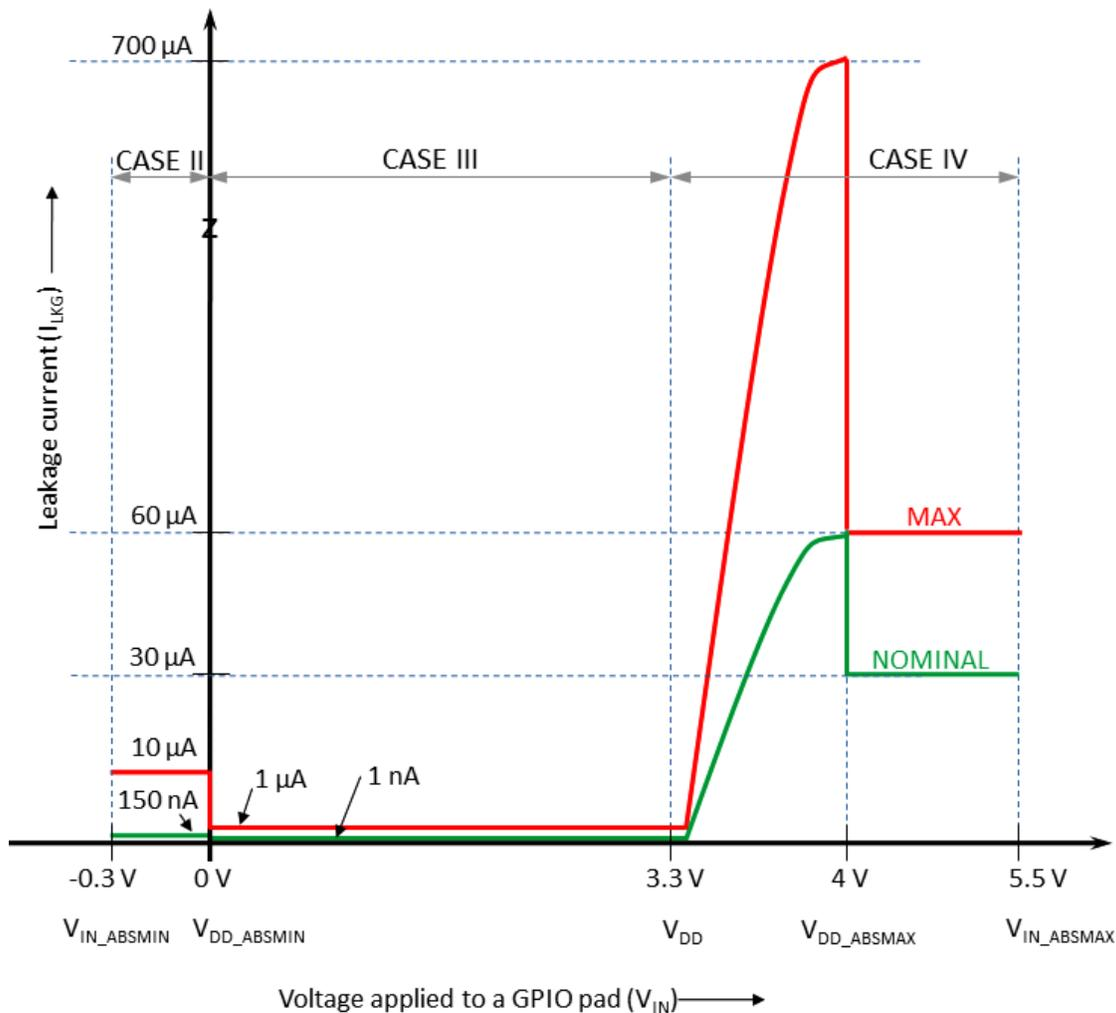
**Figure 3. Relationship Between Leakage Current and Voltage Applied to a GPIO Pin at Nominal Temperature**
