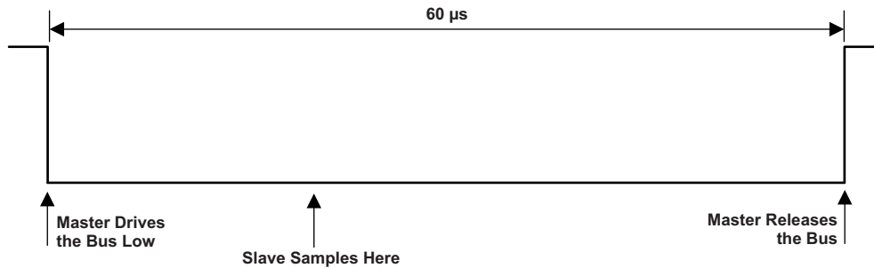
Figure 4. Write 0 Bus Timing
