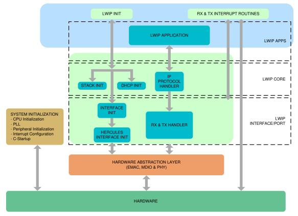
Figure 2. Software Layers With IwIP Integration
