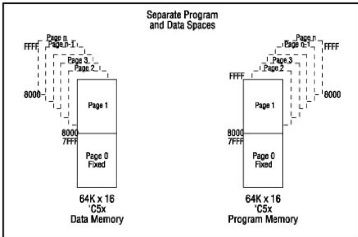
An example of a separate program and data scheme is shown above in Figure 2 with a fixed 32K page 0 in the lower half of memory and pageable 32K blocks in upper memory.
