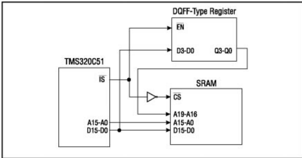
Since the bank switch requires some action from the DSP, frequent switching between banks is not very efficient. It would be best to partition tasks within a bank, and switch banks when starting new tasks. It may even be desirable to fix a certain part of the memory as nonpageable, where the task manager would run (or use internal memory). This task manager kernel could determine on which page a called function resides and swap banks accordingly.
