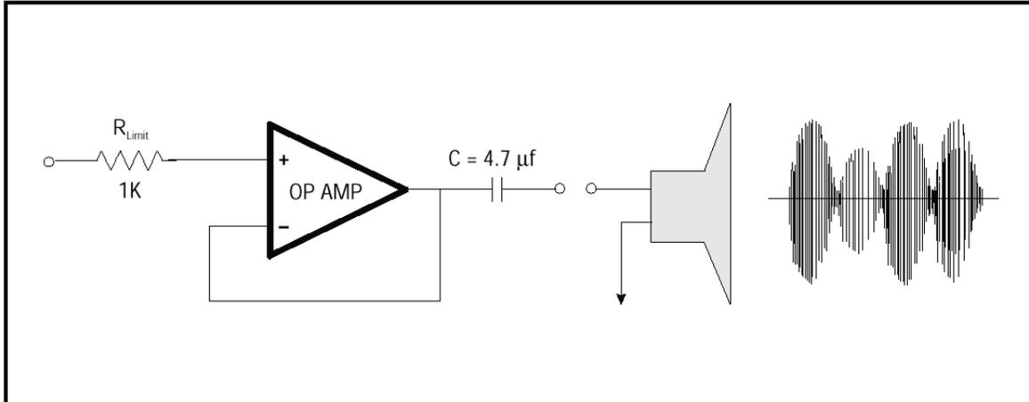
In order for the AIC to select the AUXIN+ amplified signal, you must set bit 4 of the AIC Control Register when initializing the AIC (see page B-14 of the 'C5x DSK User's Guide). The output driver can drive most 8  $\Omega$  desktop speakers.
