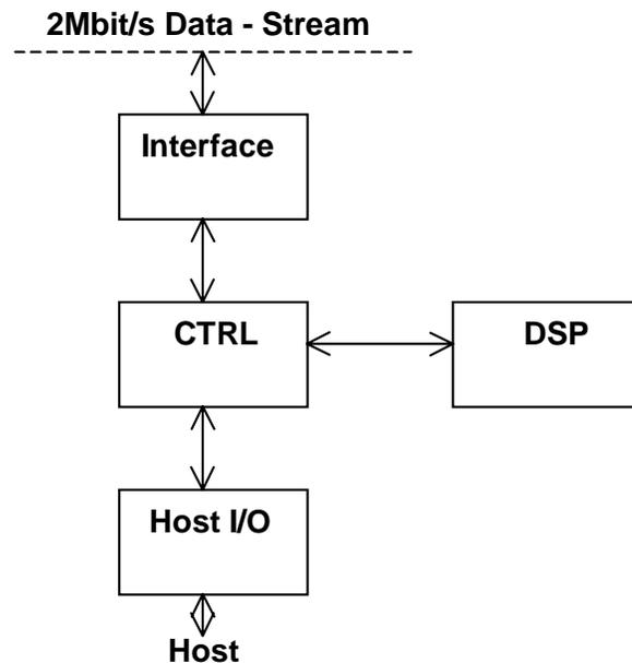
The proposed system allows the monitoring of two full-duplex voice band channels, corresponding to four time slots in the time-division multiplexed PCM frame out of the 32 simultaneously transmitted.
