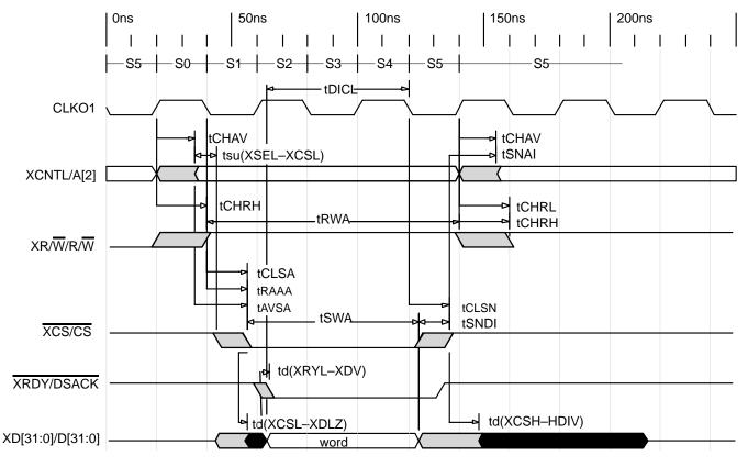
Figure 3. MC68360 (Host) Performs Read from Expansion Bus Asynchronous Host Port Interface
