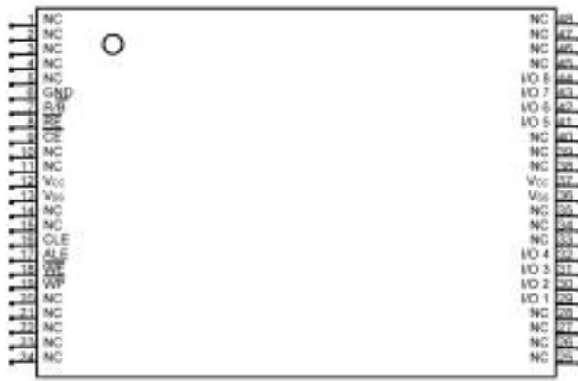
Figure 3. NAND Memory Device Package Diagram
