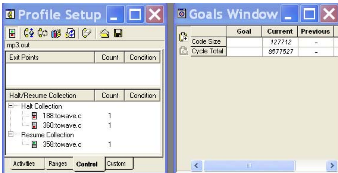
Figure 6. Profile Setup of Halt and Resume Points (left). Goals Window After First Run (right).
