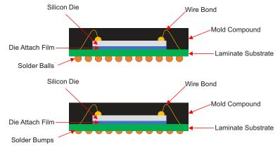
Figure 1-3. Structure of TI's Small Body nFBGA Packages
