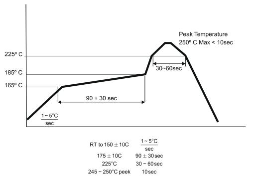
Figure 4-2. Recommended Reflow Profile of Pb-Free nFBGA Package
