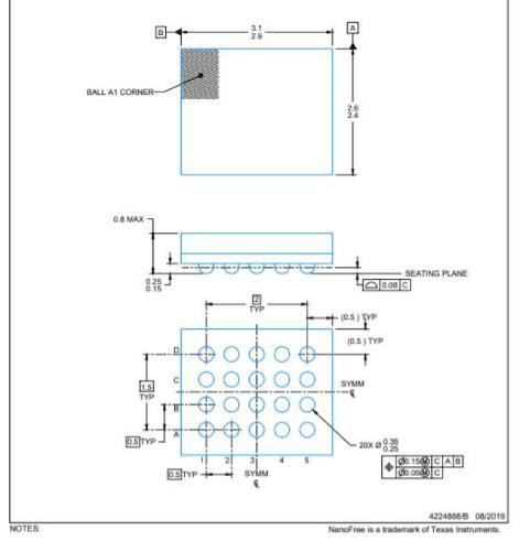
All linear dimensions are in millimeters. Any dimensions in parenthesis are for reference only. Dimensioning and tolerancing per ASME Y14.5M. This drawing is subject to change without notice. 15
