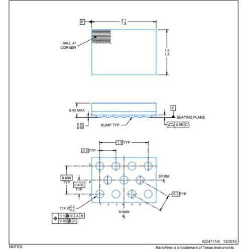
All linear dimensions are in millimeters. Any dimensions in parenthesis are for reference only. Dimensioning and tolerancing per ASME Y14.5M. This drawing is subject to change without notice. 1.
