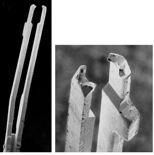
Figure 6-2. Pinch Contact for Solder Ball
