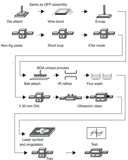
Figure 1-4. nFBGA Package Assembly Flow
