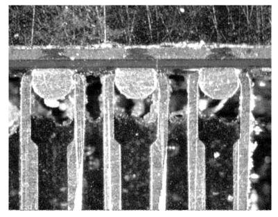
Figure 6-3. Contact Area on Solder Ball
