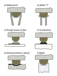
Figure 6-1. Approaches for Contacting the Solder Ball
