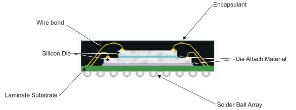
Figure 1-2. Structure of TI's nFBGA Package
