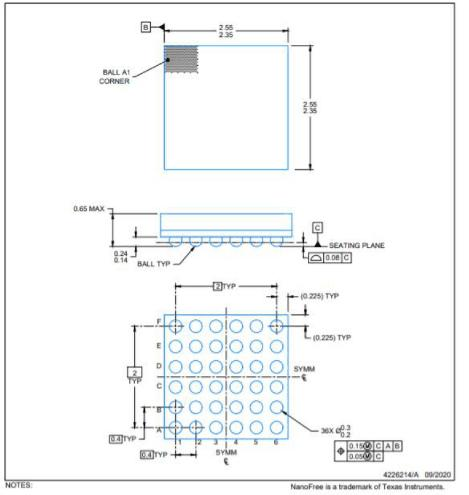
1. All linear dimensions are in millimeters. Any dimensions in parenthesis are for reference only. Dimensioning and tolerancing ner ASME V14 5M
