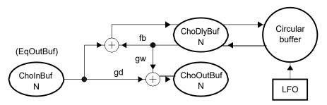
Figure 9. Block-Processing Diagram for Chorus Module
