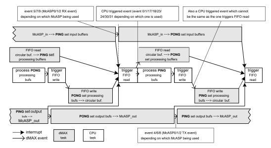
Figure 19 illustrates how the PING-PONG buffer scheme works.
