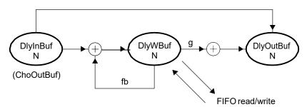
Figure 11. Block-Processing Diagram for Delay Module
