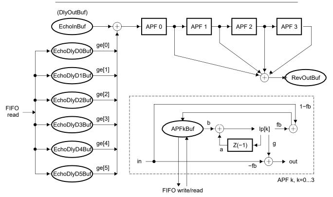
Figure 13. Block-Processing Diagram for Reverb Module
