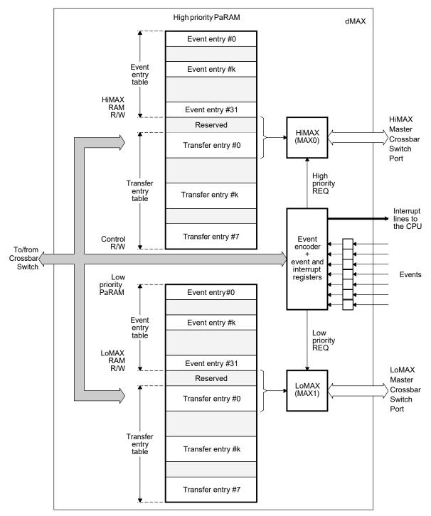
Figure 2. dMAX Block Diagram
