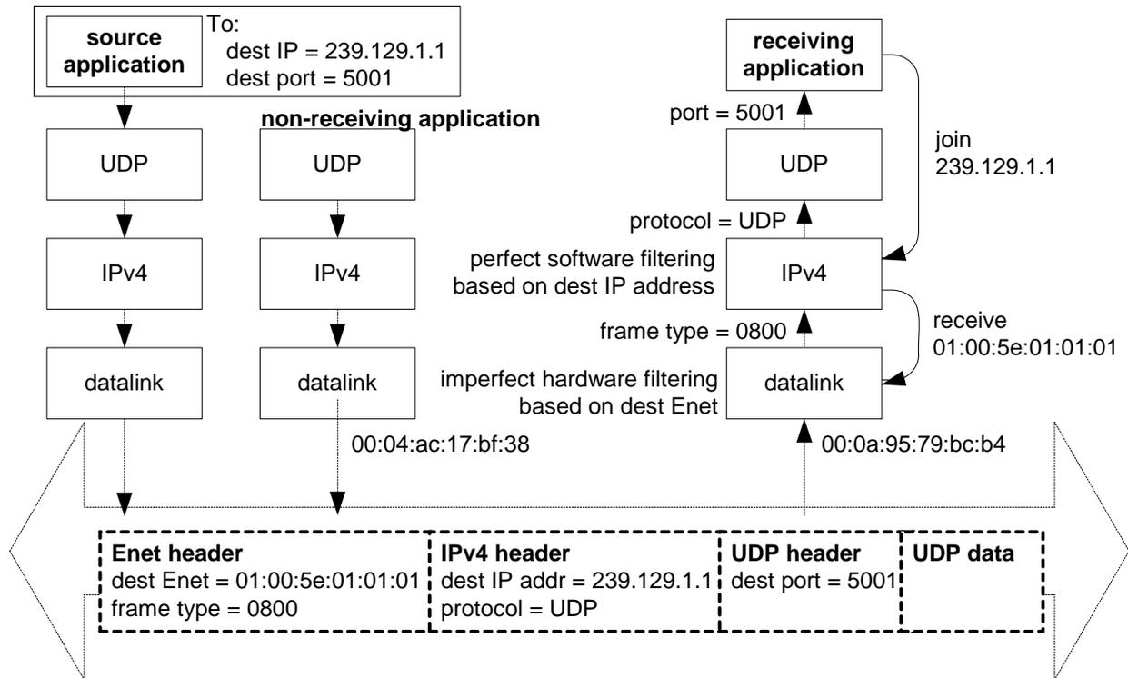
Similarly, to be able to send data to a multicast group, a host must create a UDP socket with the same port and group address as the listening socket. The same socket cannot be used to send and receive packets, since the IP standard forbids packets from having a multicast address as the source address.
