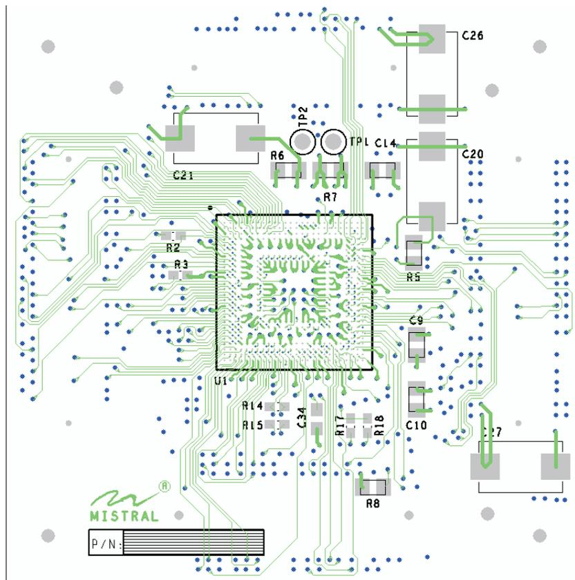
**Figure 26. Layer 1 – Signal - Top Copper – Area Around The OMAP25x**
