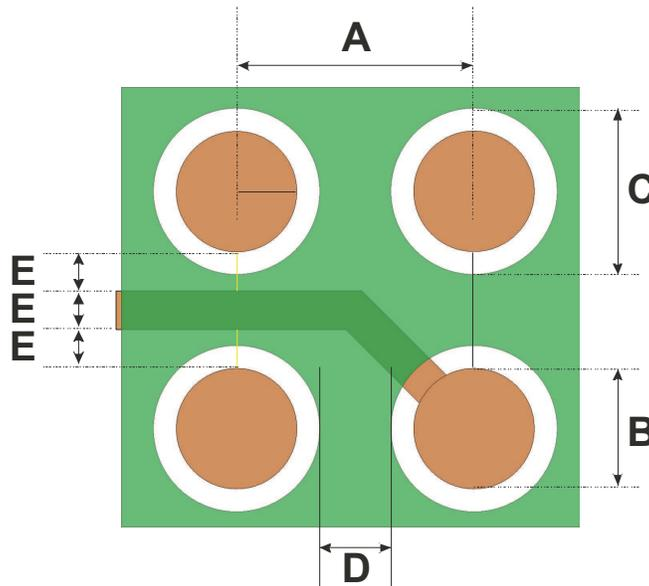
**14 PCB Dimensions for 0.5mm Pitch with Via**
