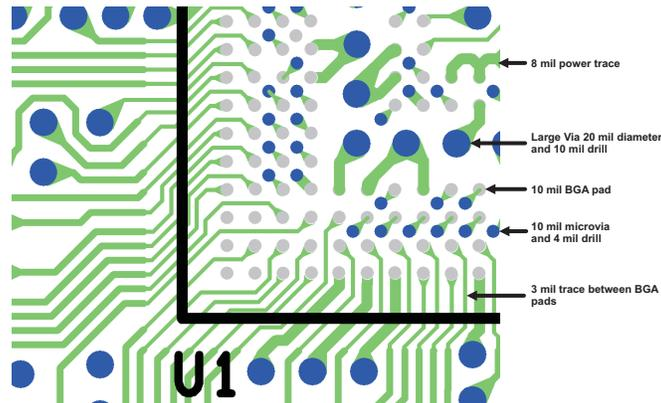
The microvia only goes between layer one and layer two on this design. There are no stacked vias. The small vias are from layer two to layer one. The large vias are through vias from top to bottom.
