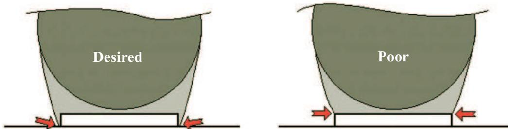
With proper stencil design, proper paste deposition, proper paste formulation and correct reflow temperatures, the solder will wet the solder ball and adhere to the edges of the copper pad resulting in a very strong and robust joint that can withstand the rigors of today’s consumer products.
