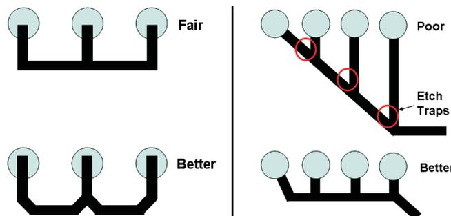
Small BGA pads do not have much solder and depend on uniform heating for a good joint. Here are some tips to ensure that traces and vias do not serve as heatsinks.
