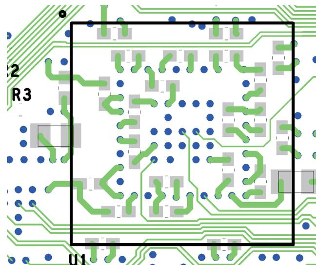
The majority of the components within the U1 outline (which is not physically present on the bottom silkscreen) are bypass capacitors.
