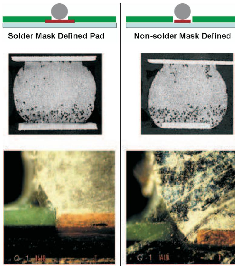
However, there are some companies that swear by SMD pads claiming that the greater copper area (of the pad) and the solder-mask overlap create better adhesion strength to the fiber/glass laminate. They claim that flexing and bending during accelerated thermal cycling testing causes a weak link where the pad attaches to the PCB and could be the main failure location, as opposed to the typical solder fracture which dominates the NSMD pad.
