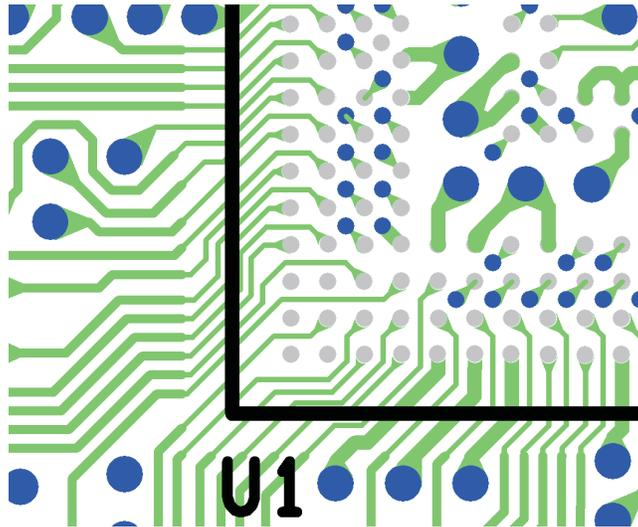
Note that this viewer shows the individual traces used to approximate the teardrop trace exit from the pads and vias.
