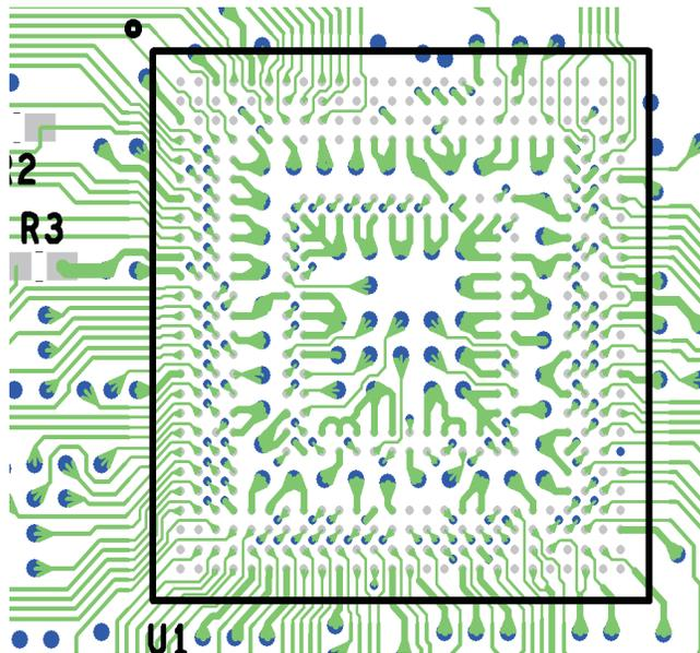
**Figure 28. Layer 1 – Top Copper – Close Up View and Measurements**
