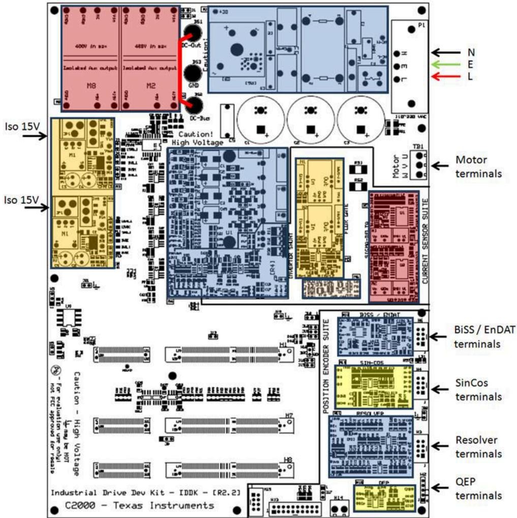
Figure 8-2. Powering IDDK From an AC Source
