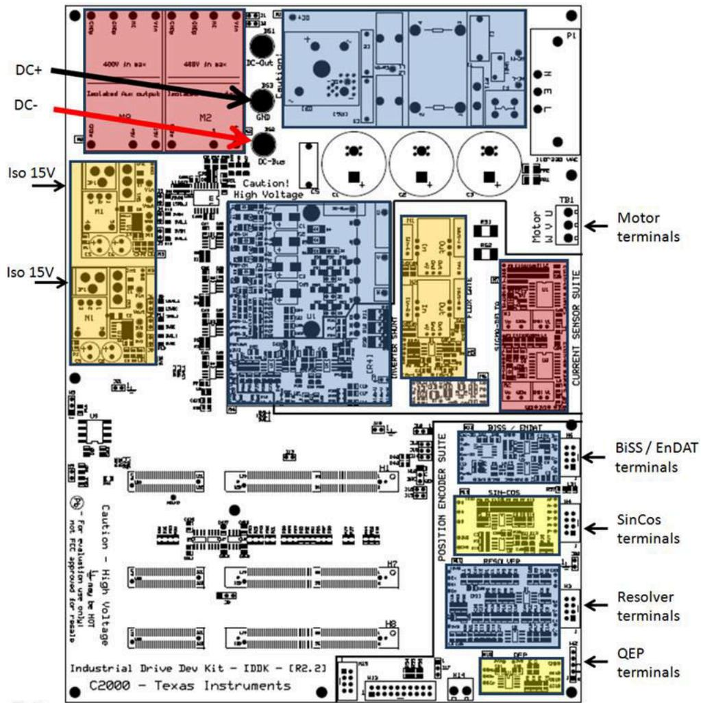
**Figure 8-1. Powering IDDK From External DC Power Supply**
