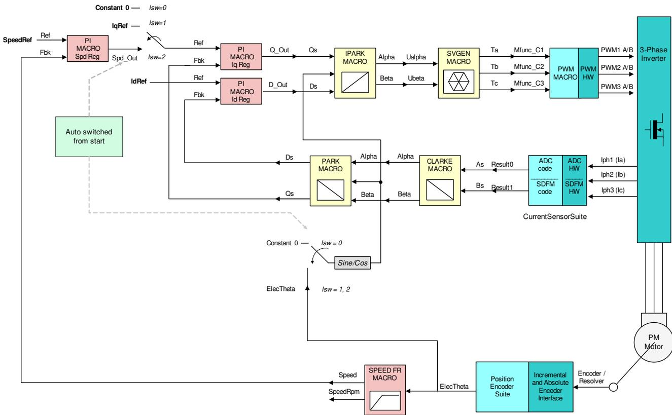
Figure 9-13. Level 4 - Incremental System Build Block Diagram
