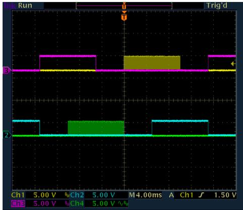
**Figure 6 The PWM outputs , PWM 1 (Yellow) , PWM 2 (Pink) and PWM 5 (Green), PWM 6 (Blue)**
