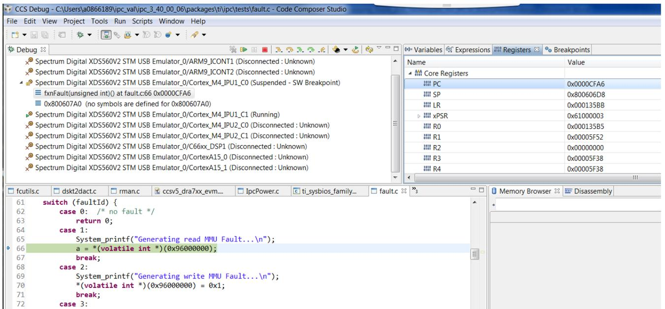
Use this technique at any time after booting the remote core to see what a PC address corresponds to. It will display the line that caused the error. This may, however, prevent proper execution because the registers and call stack won't have proper values.
