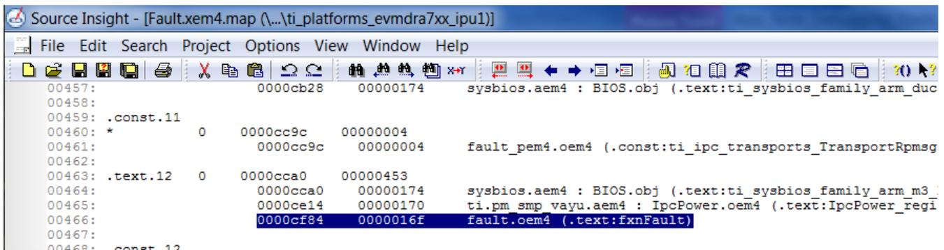
Alternatively, use CCS to see the location of the fault. If CCS was already connected to the remote core before the fault happened, the core will have halted in the abort function. From here, directly set the PC address and see the line that caused the fault:
