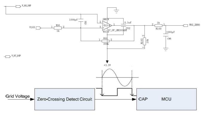
Figure 9. AC Waveform Frequency Detection Circuit
