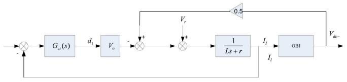
Figure 15. Closed-Loop Diagram
