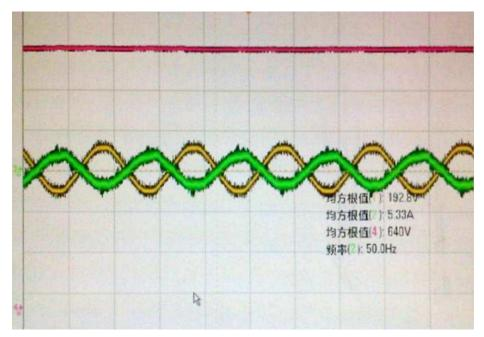
Figure 23. Current and Voltage Waveform in Inverter Mode
