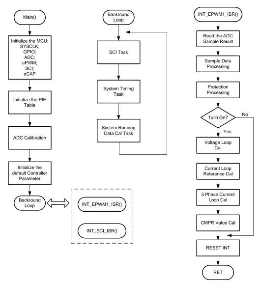
Figure 12. Software Main Process Flow
