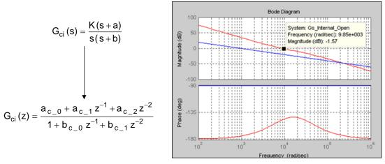
Figure 17. Current Loop Controller Analysis
