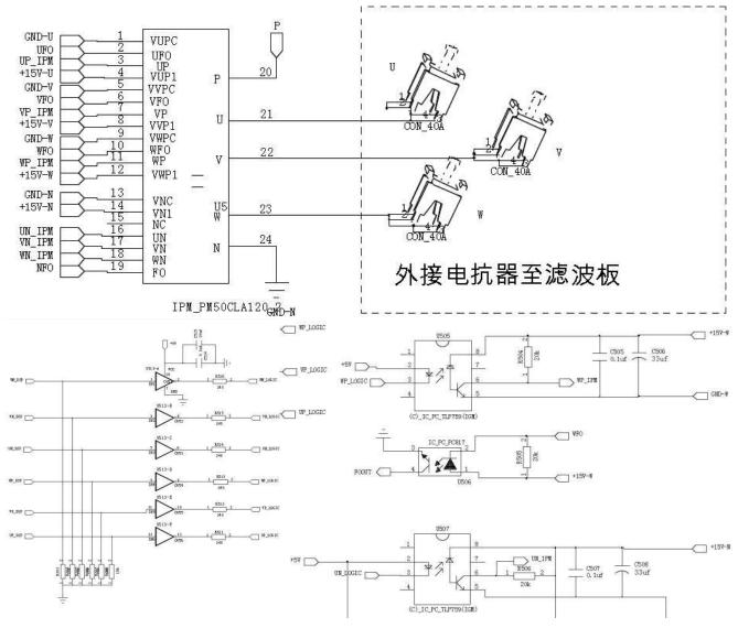
Figure 5. 3-Phase Bridge Driver Circuit
