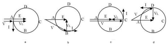
Figure 11. Current and Voltage Phase Relationship
