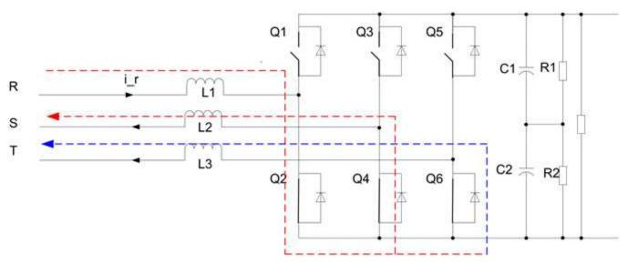
Figure 3. Circuit Analysis for Arm On
