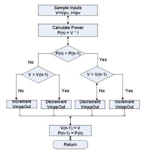
Figure 20. MPPT Algorithm Flow
