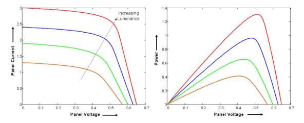
Figure 18. V-I Curves for Solar Cell
