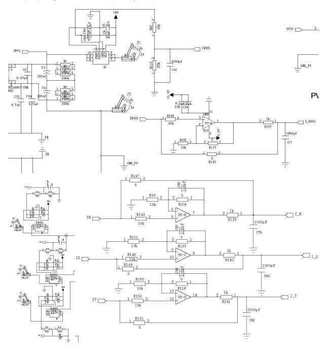
Figure 8. Current Signal Sample Circuit
