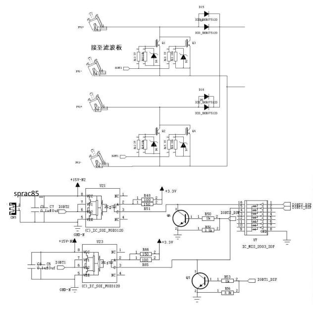
Figure 6. Boost Driver Circuit
