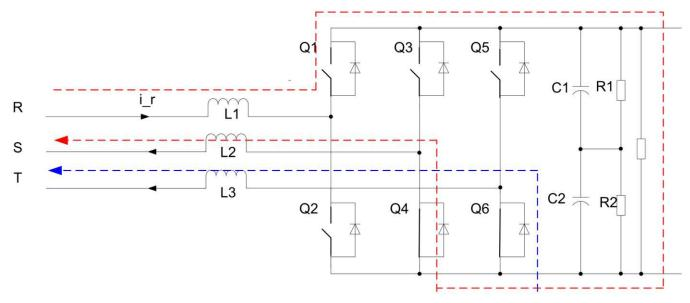
Figure 4. Circuit Analysis for Arm Off
