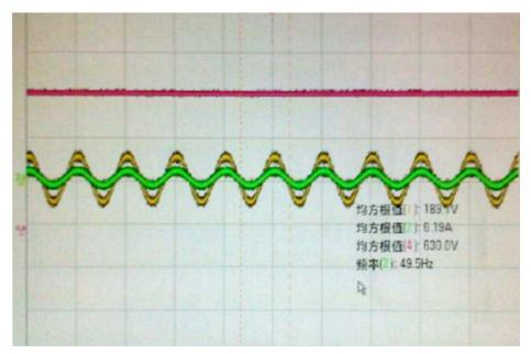
Figure 21. Current and Voltage Waveform in PFC Mode
