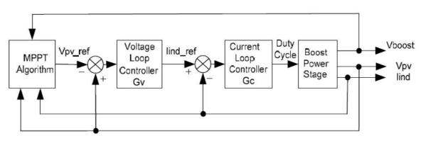
Figure 19. DC-DC Control Loop Diagram
