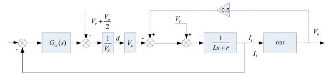
Figure 16. Simplified Control Loop
