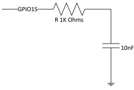
**Figure 1. Hardware Connections**
