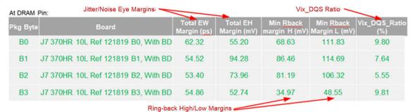
Figure 3-12. LPDDR4 Simulation Results for Write
