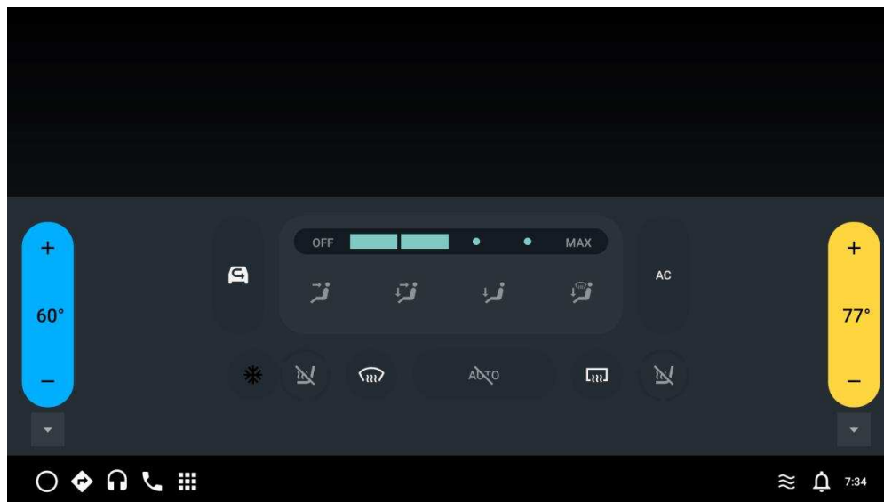
Figure 4. Climate Control Interface for Automotive Configuration (allowing you to adjust temperature, fan speed and direction, seat warmers, and so forth)
