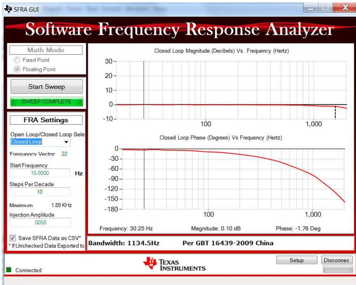
Figure 37. SFRA Closed Loop Bode Plots of the Current Loop Showing Magnitude and Phase Angle
