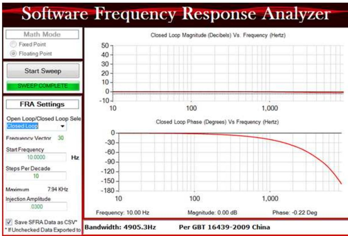
Figure 39. SFRA Closed Loop Bode Plots of the Current Loop - Current Feedback With High SNR
