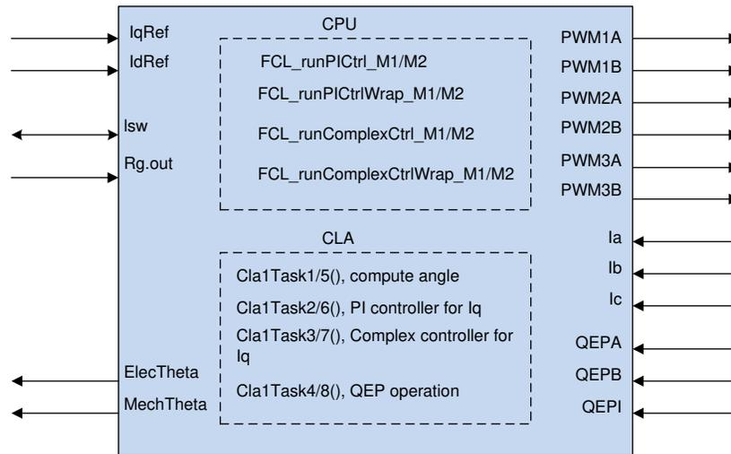
**Figure 3. Fast Current Loop Block Diagram**
