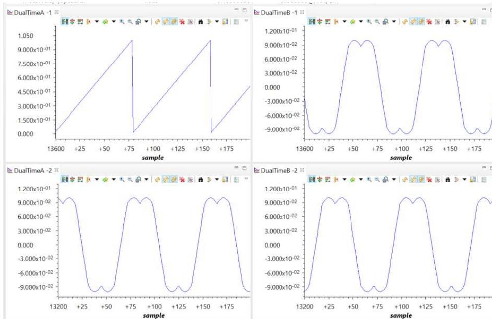
Figure 20. Voltage Vector Angle and SVGEN Ta, Tb, and Tc Using Graph Tool
