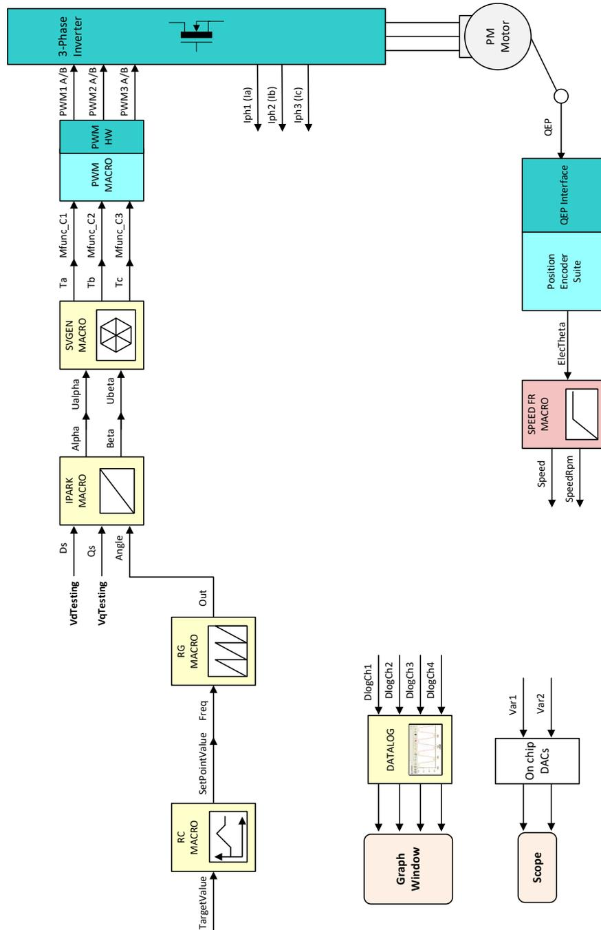
Figure 22. Level 2 Block Diagram
