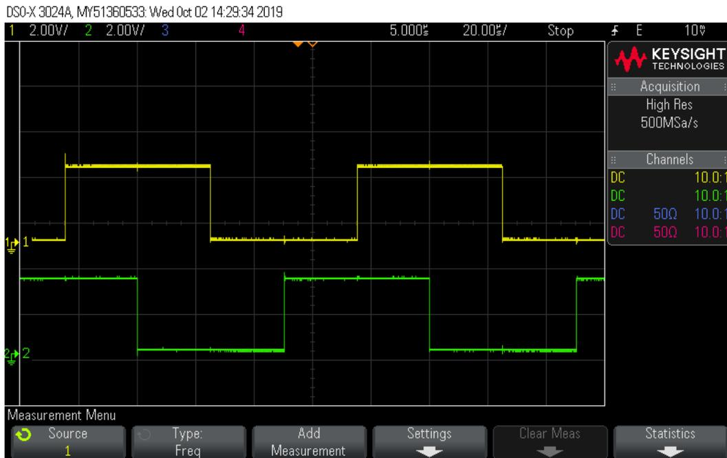
**Figure 19. PWM\_UH of Motor 1 and Motor 2 on Scope Plots**
