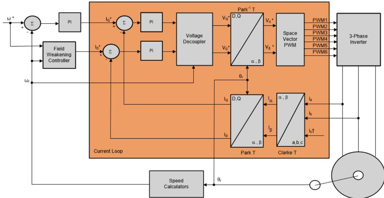
Figure 1. Basic Scheme of FOC for AC Motor
