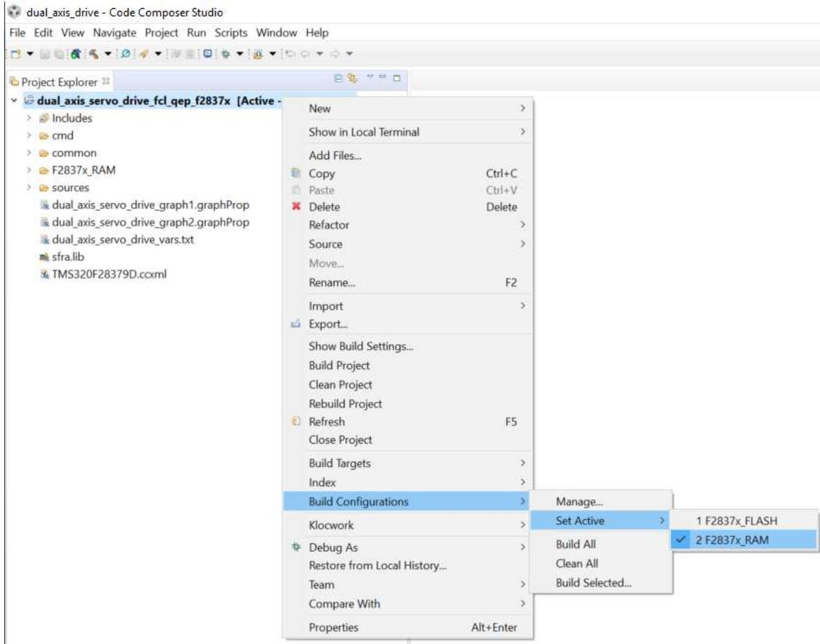
**Figure 12. Selecting the F2837x\_RAM Configuration**
