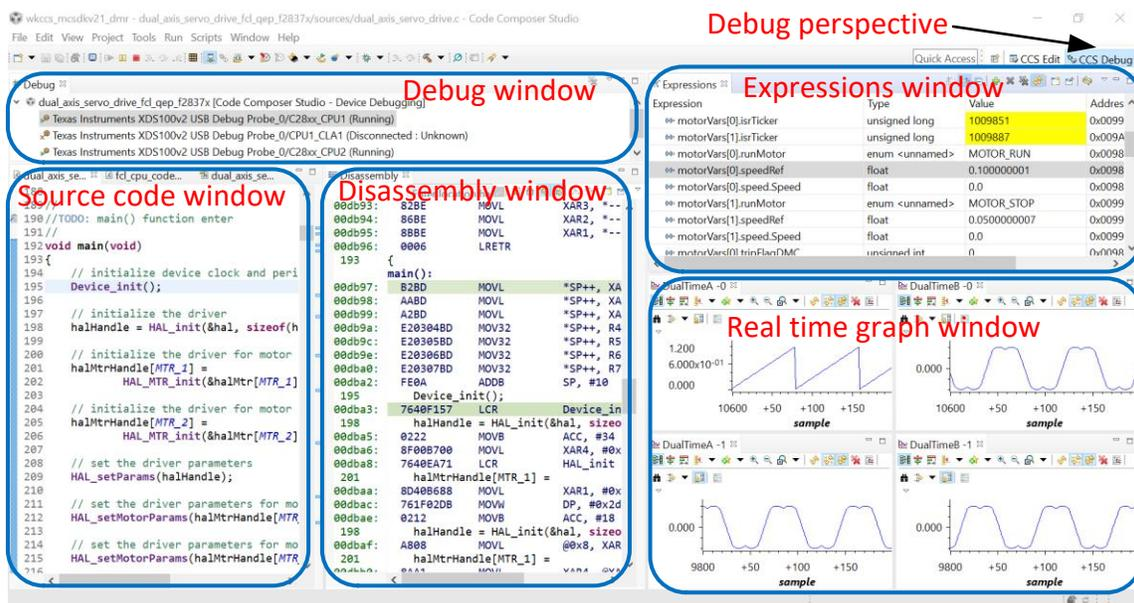
Figure 17. CCS IDE Showing Debug Perspective
