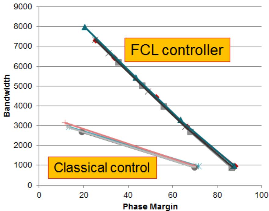
Figure 40. Plot of Gain Cross over Frequency vs Phase Margin as Experimentally Obtained
