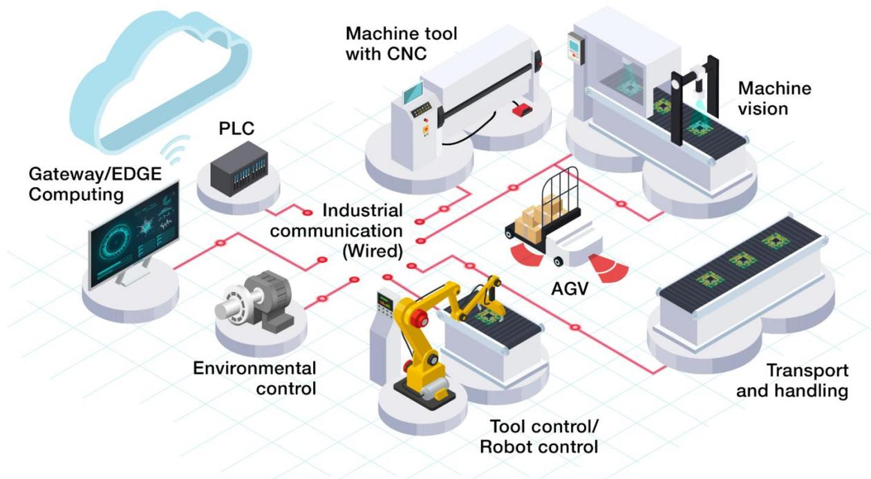
**Figure 2. Factory floor setting**
