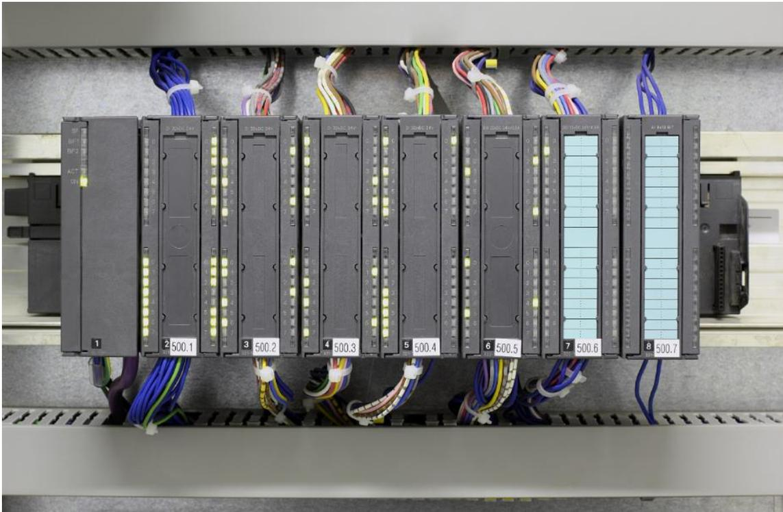
Figure 1. A typical PLC
