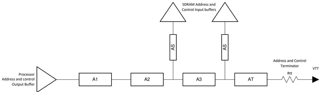
**Figure 2-6. ADDR\_CTRL Topology for Two DDR4 SDRAM Devices**
