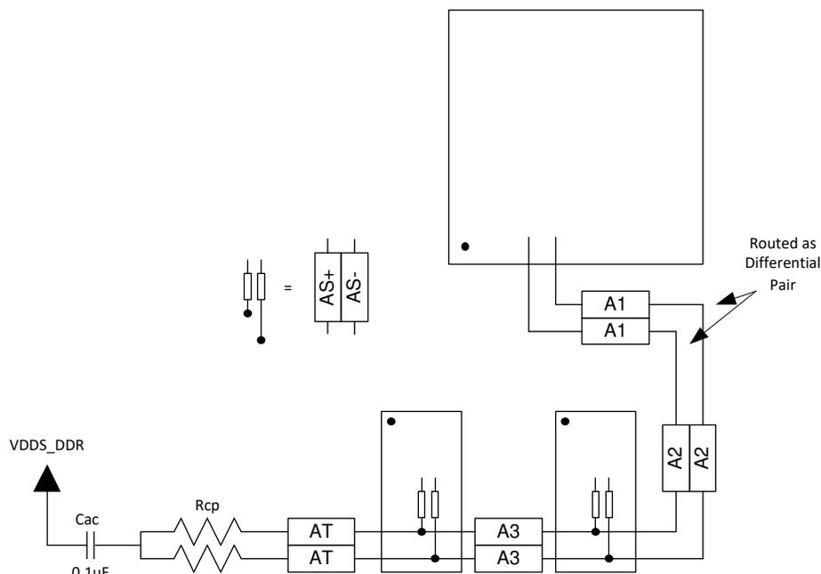
**Figure 2-7. CK Routing for Two DDR4 SDRAM Devices**
