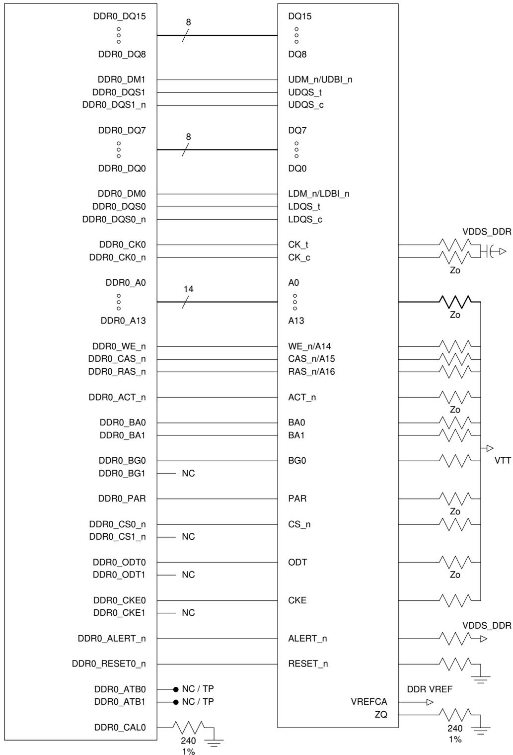
**Figure 2-1. 16-Bit, Single-Rank DDR4 Implementation Using x16 SDRAM**
