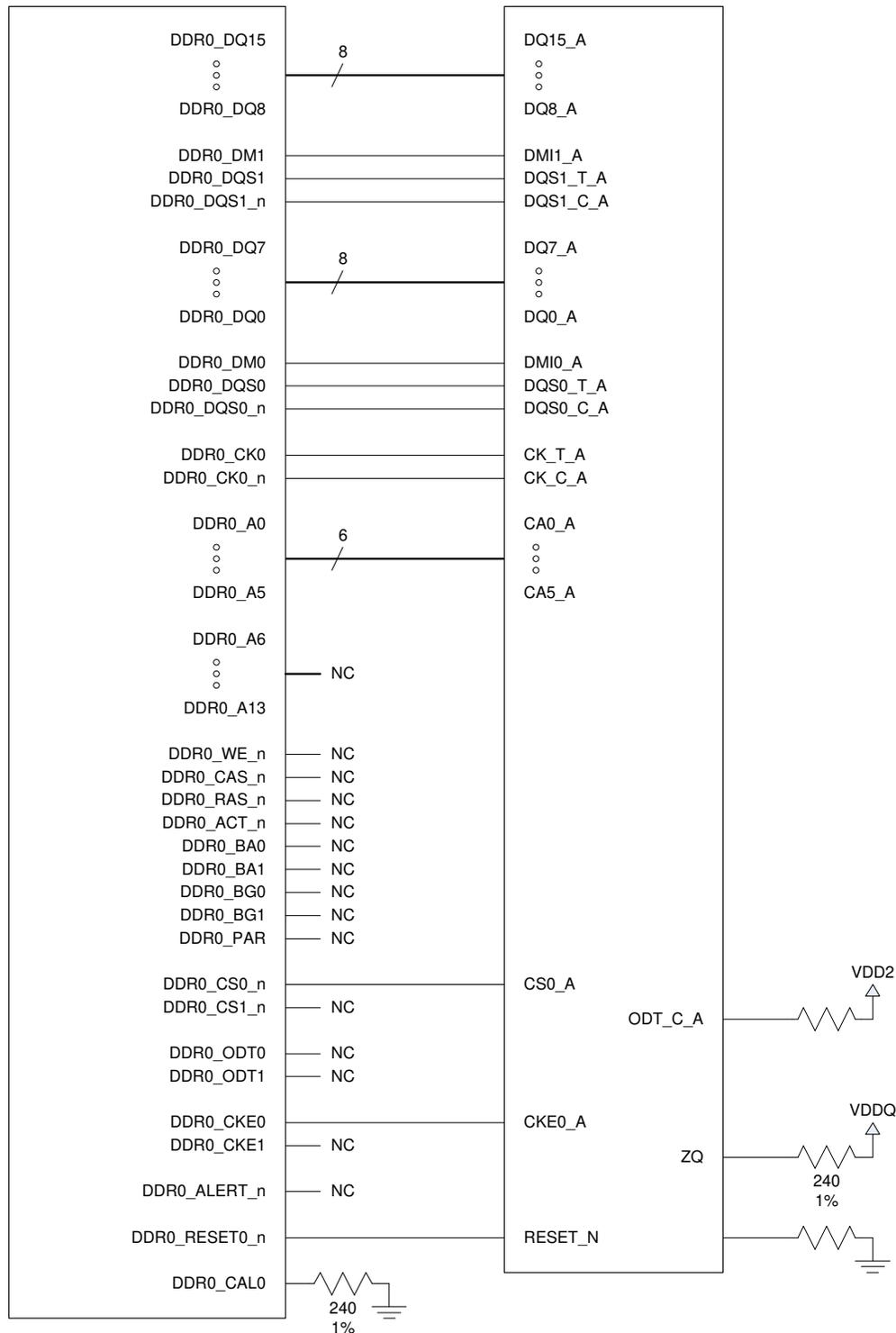
**Figure 3-1. 16-Bit, Single-Rank, Single Channel LPDDR4 Implementation**
