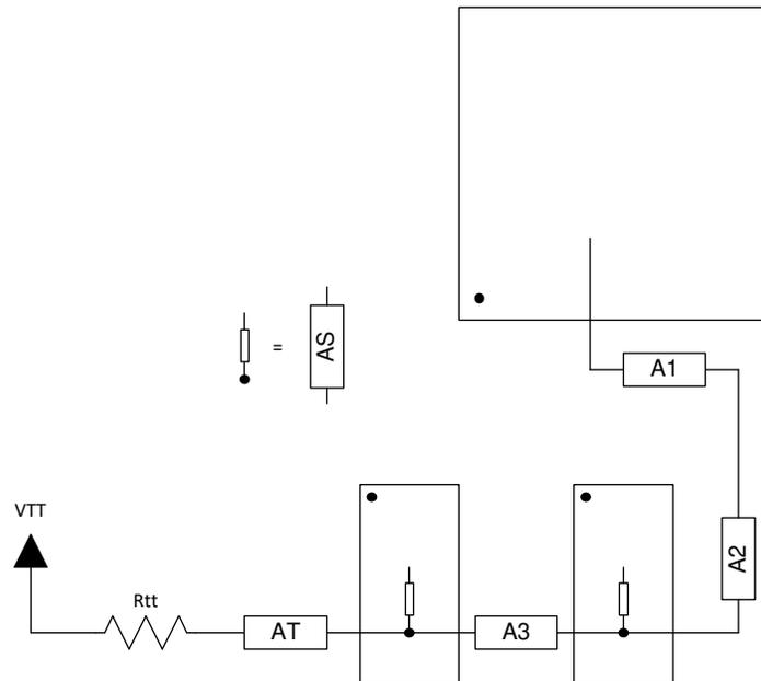
**Figure 2-8. ADDR\_CTRL Routing for Two DDR4 SDRAM Devices**
