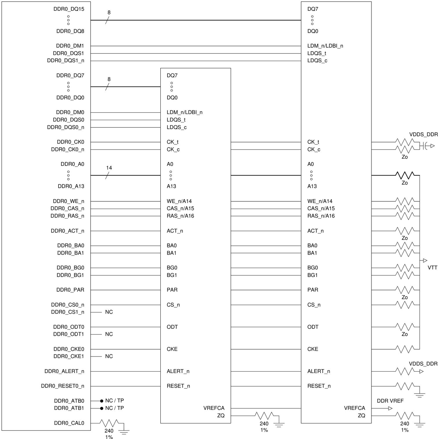
Figure 2-2. 16-Bit, Single-Rank DDR4 Implementation Using x8 SDRAMs
