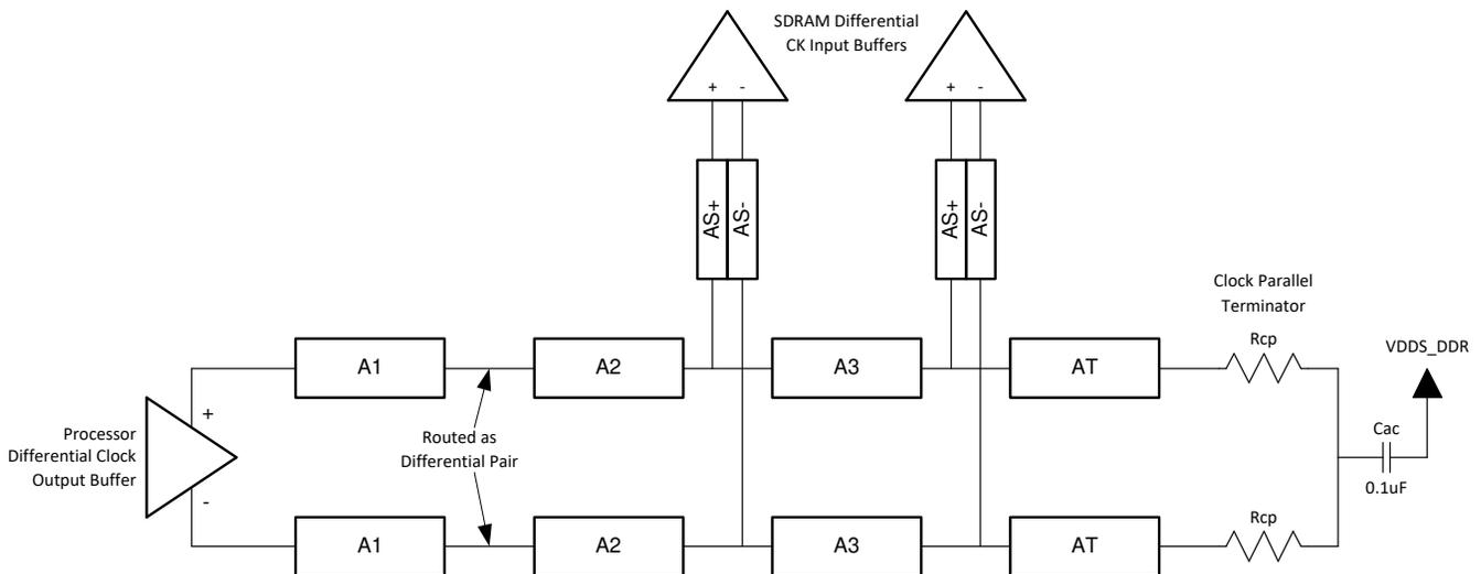
Figure 2-5. CK Topology for Two DDR4 SDRAM Devices
