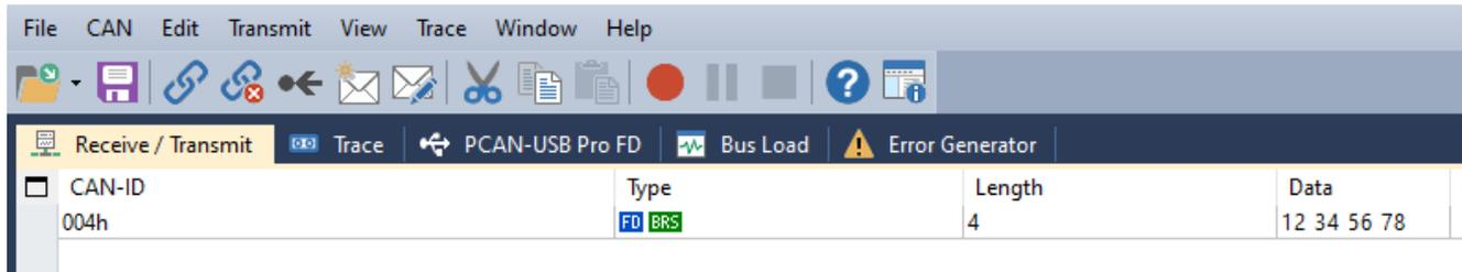
Figure 3-2. Output of Bus-Monitoring Tool for `mcan_ex1_loopback.c`
