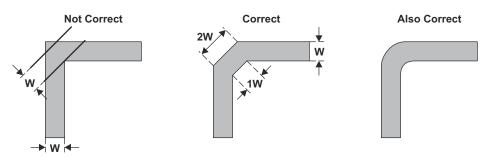
Figure 4-10. Proper Trace Signal Routing
