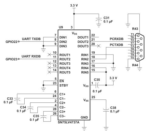
Figure 3-6. Typical RS-232 Transceiver
