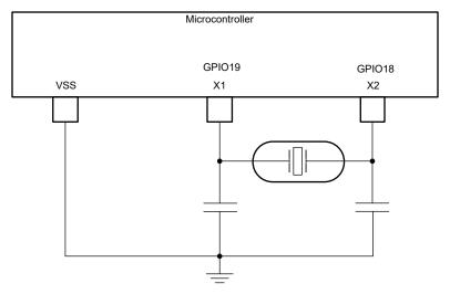
Figure 3-13. External Crystal Circuit
