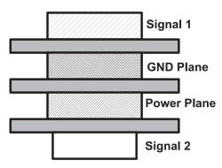
Figure 4-1. Layer Stack-Up for 4-Layer Board
