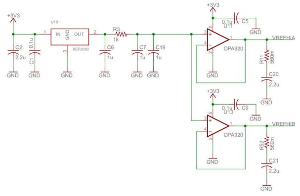
Figure 3-7. Reference Circuitry for External Analog Reference
