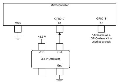
Figure 3-15. External Oscillator Circuit
