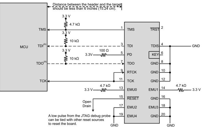
Figure 3-16. Typical JTAG Probe Connections
