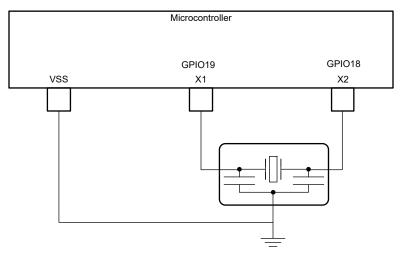
Figure 3-14. External Resonator Circuit
