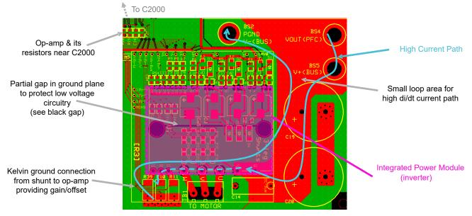
Figure 4-6. Power Electronics on Board Layout
