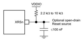
Figure 3-12. External Reset Circuit
