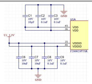
Figure 3-9. Decoupling Capacitors on VDD Pins
