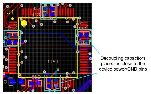
Figure 4-5. Decoupling Capacitors on Board Layout
