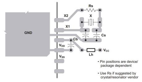
Figure 4-4. Recommended Oscillator Layout
