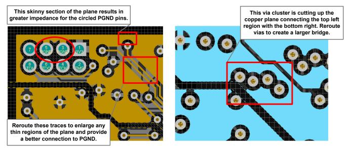
Figure 4-8. Examples of Cut-Up Ground Planes
