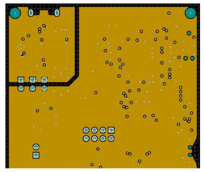
Figure 4-7. Ground Plane on LaunchPad
