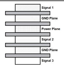
Figure 4-2. Layer Stack-Up for 6-Layer Board
