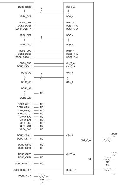
Figure 3-1. 16-Bit, Single-Rank, Single Channel LPDDR4 Implementation
