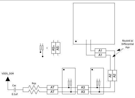
Figure 2-7. CK Routing for Two DDR4 SDRAM Devices
