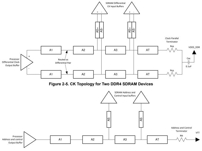
Figure 2-6. ADDR\_CTRL Topology for Two DDR4 SDRAM Devices
