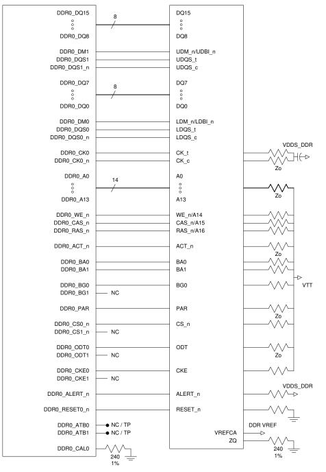
Figure 2-1. 16-Bit, Single-Rank DDR4 Implementation Using x16 SDRAM
