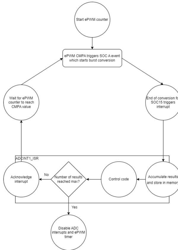
**Figure 4-1. SoC Flow Diagram for Oversampling**
