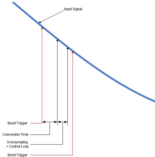
**Figure 4-2. Timings for Sampling a Signal**
