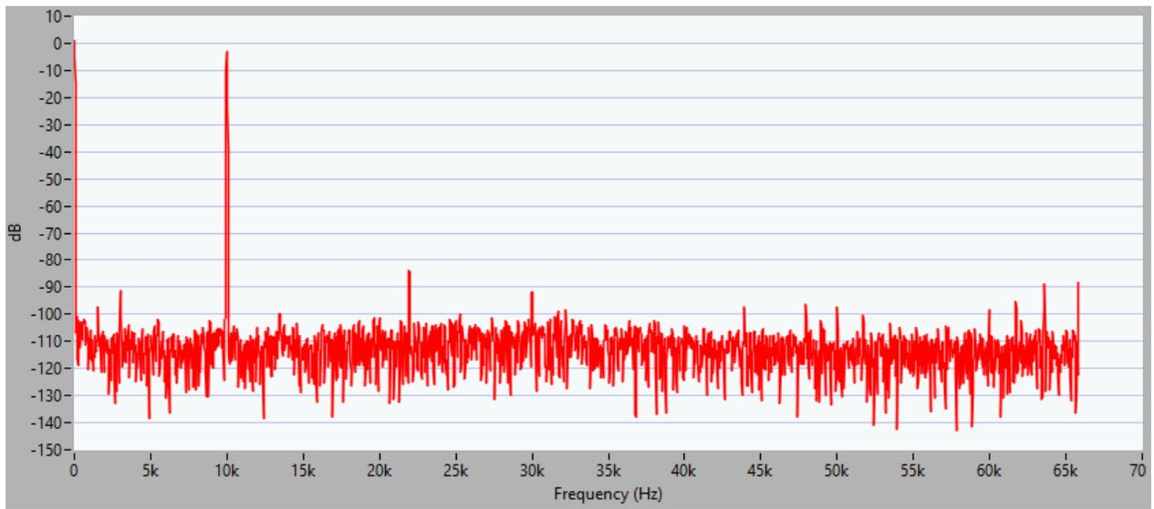
**Figure 5-4. 8X Oversampling FFT Plot**
