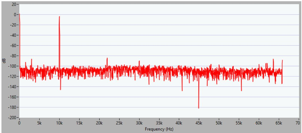
**Figure 5-3. 4X Oversampling FFT Plot**
