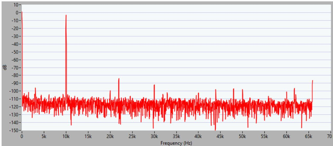
**Figure 5-5. 16X Oversampling FFT Plot**
