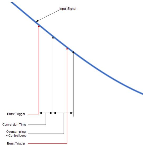
**Figure 4-3. Incorrect Timings for Sampling a Signal**
