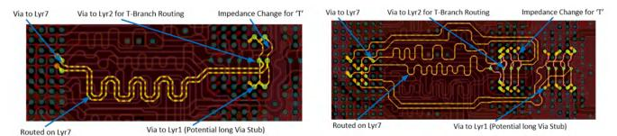
Figure 3-7. Example LPDDR4 Clock and CA Routing
