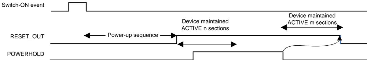
Figure 6. Typical POWERHOLD Use Case
