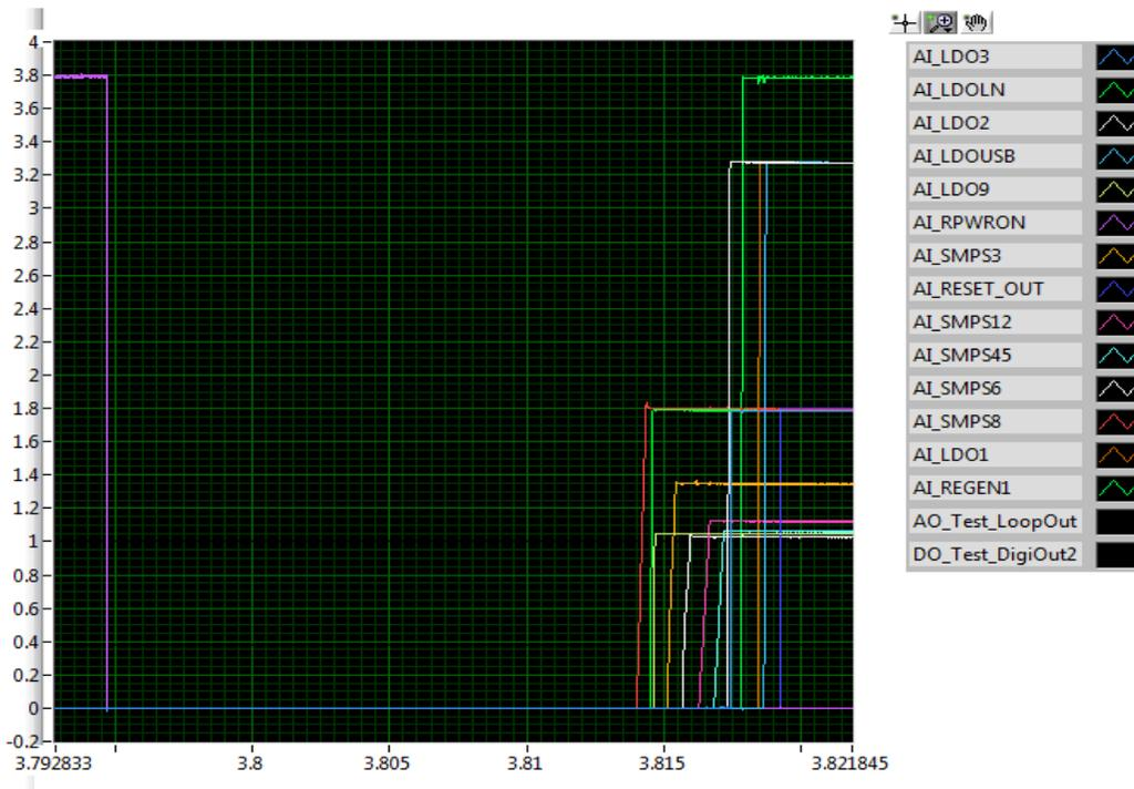
Figure 4. ON Request Using RPWRON
