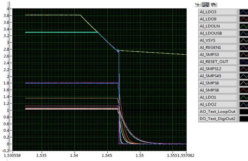
Figure 12. OFF Request by Removal of Supply Voltage (VSYS\_LO)
