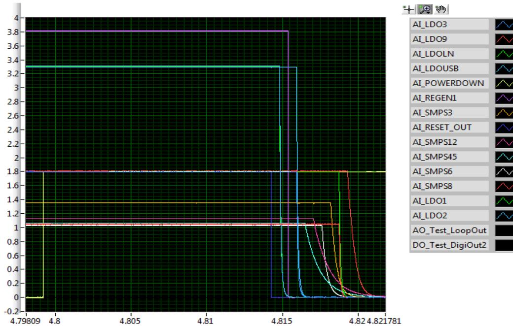
Figure 9. OFF Request Using POWERDOWN
