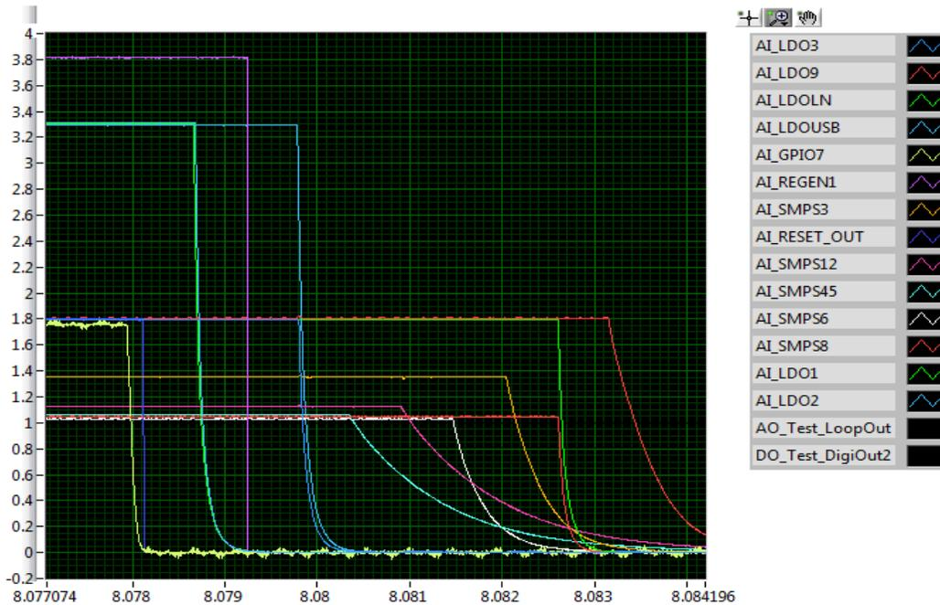
Figure 13. OFF Request Using POWERHOLD
