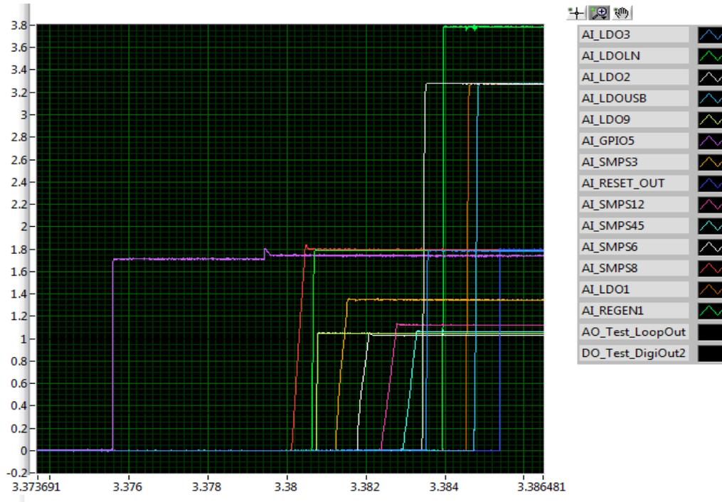
Figure 5. ON Request Using GPIO\_5 Interrupt
