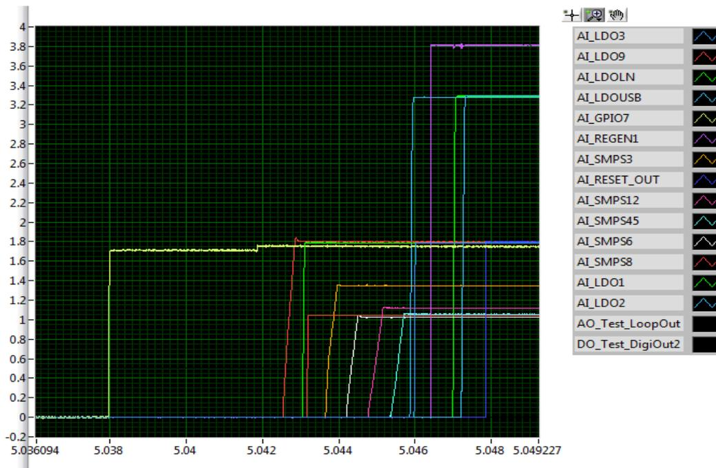
Figure 7. ON Request Using POWERHOLD
