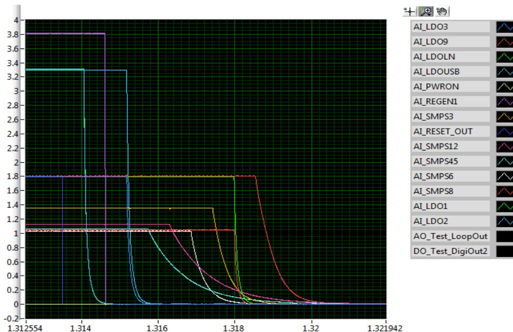
**Figure 8. OFF Request Using Long Key Press (PWRON)**
