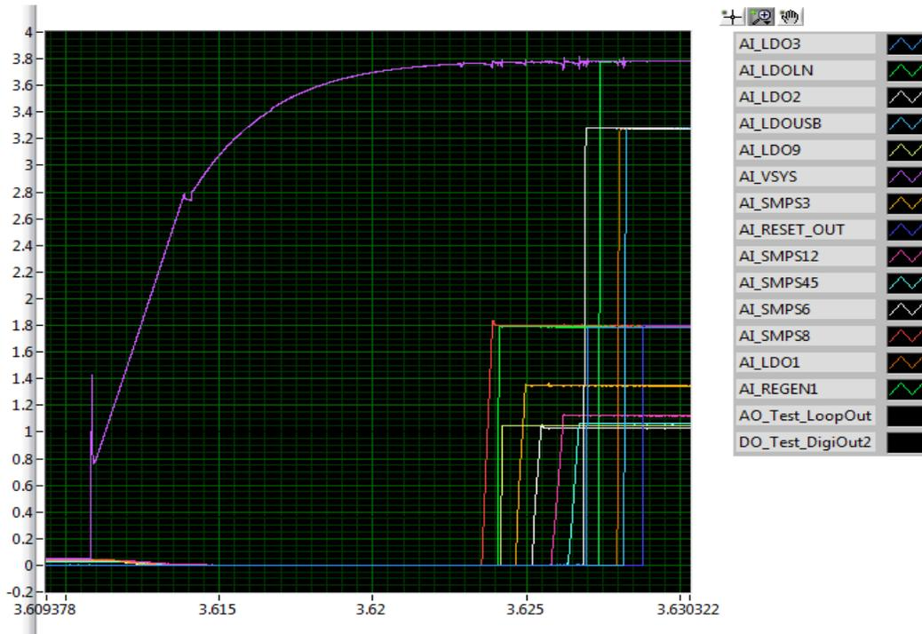
Figure 1. ON Request using First Supply Detection (VSYS\_HI)
