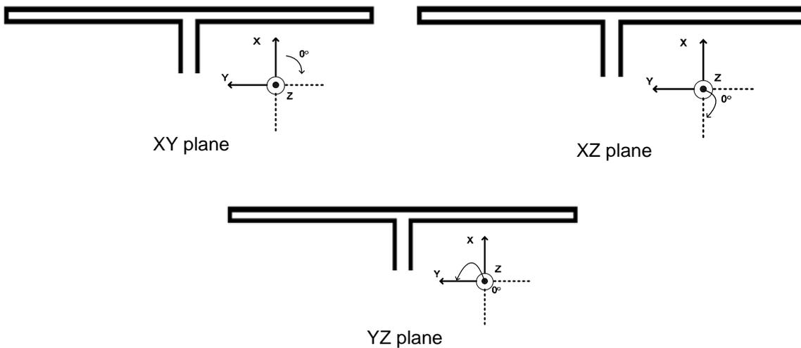
**Figure 4: How to relate the antenna to the radiation patterns.**
