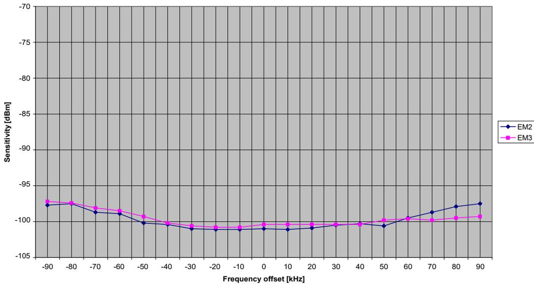
Figure 10. Sensitivity at PER 20% versus Frequency Offset
