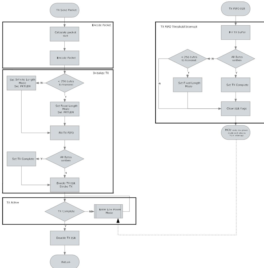
Figure 12. TX Flow Diagram
