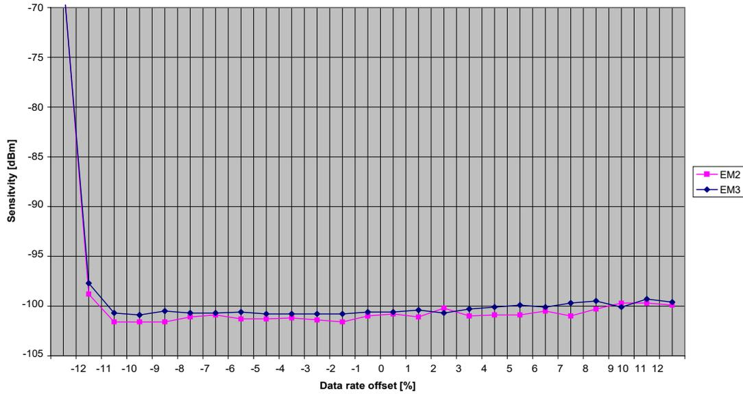
Figure 8. Sensitivity at PER 20% versus Data Rate Offset
