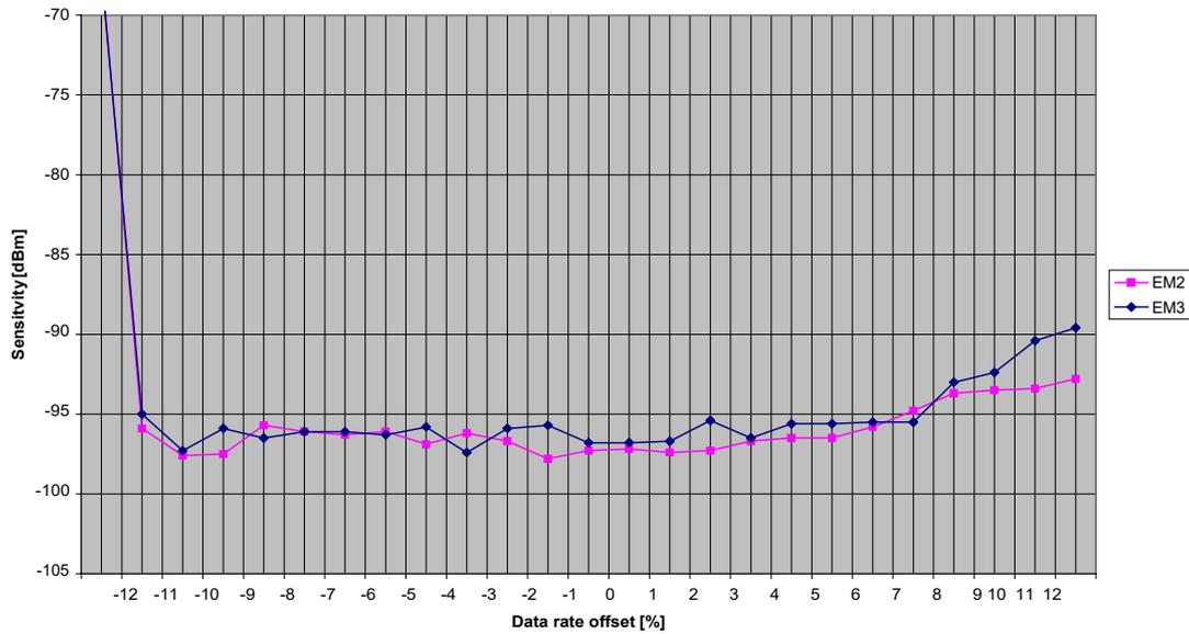
Figure 9. Sensitivity at PER 1% versus Data Rate Offset
