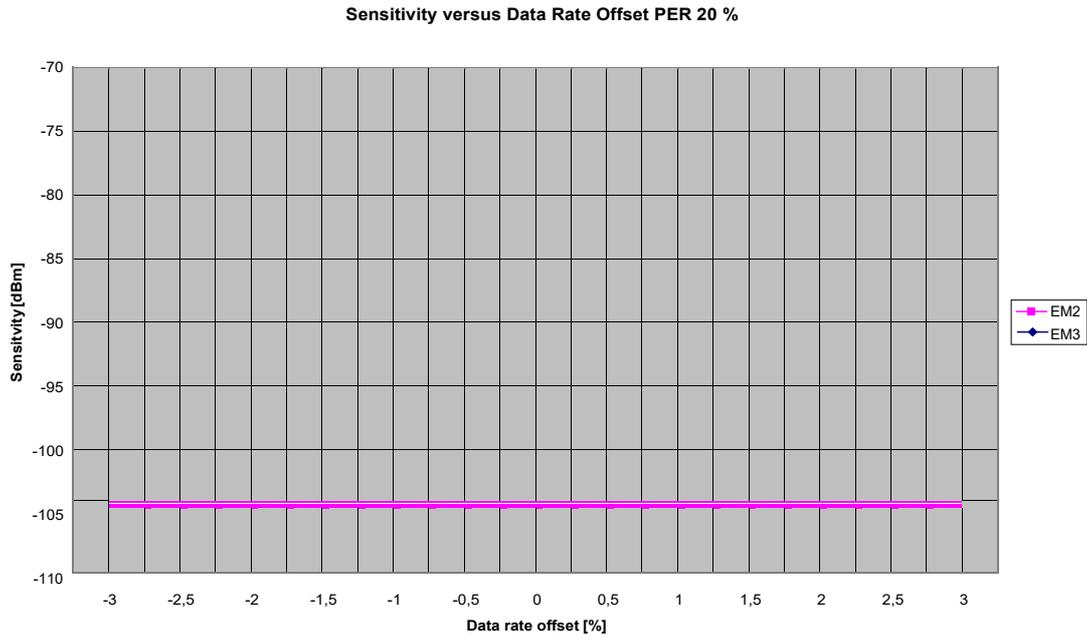
**Figure 3. Sensitivity at PER 20 % versus Data Rate Offset**
