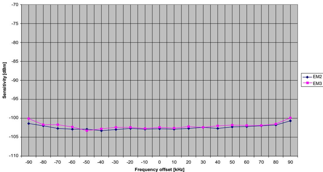
Figure 6. Sensitivity at PER 1 % versus Frequency Offset
