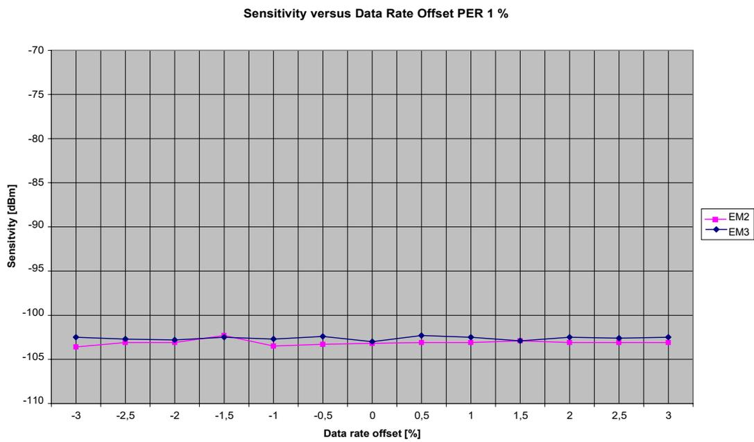
**Figure 4. Sensitivity at PER 1% versus Data Rate Offset**
