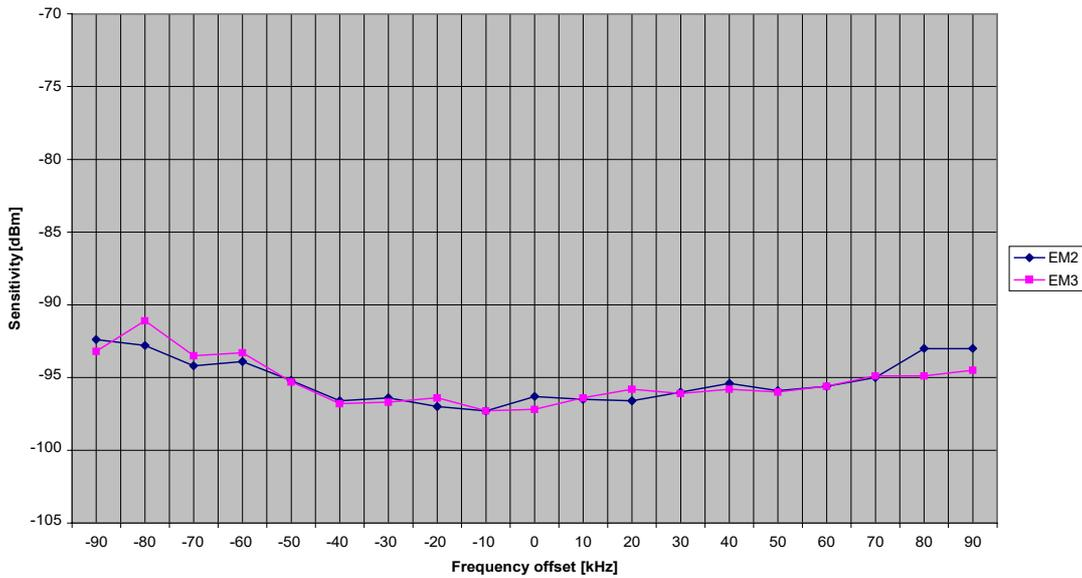
Figure 11. Sensitivity at PER 1% versus Frequency Offset
