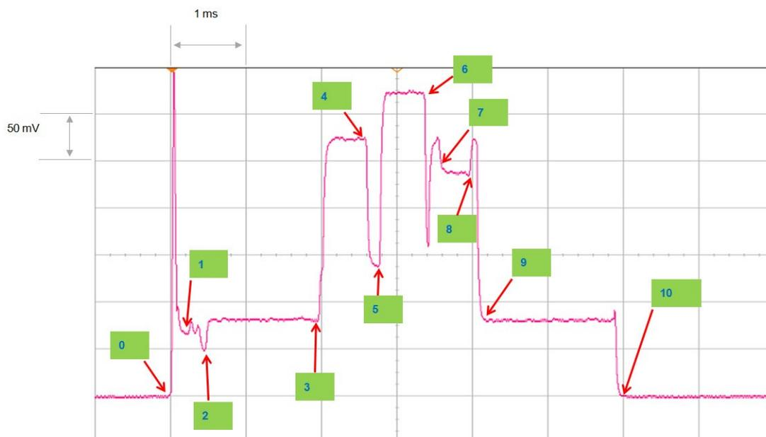
Figure 10 – Current Consumption Measurement Plot on Operation1
