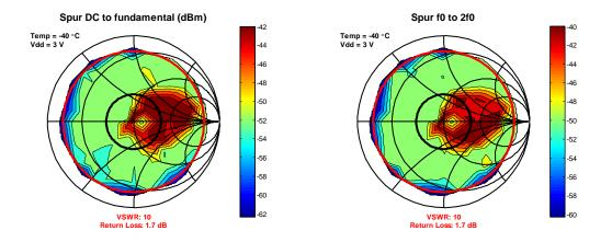
Figure 4.3. Spurious Frequency Components vs. Load Impedance at SMA Connector at -40°C, 3 V. TXPOWER = 0xFE.
