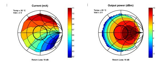
Figure 4.1. Current (left) and Output Power (right) vs. Load Impedance at SMA Connector at 25°C, 3 V. TXPOWER = 0xFE.
