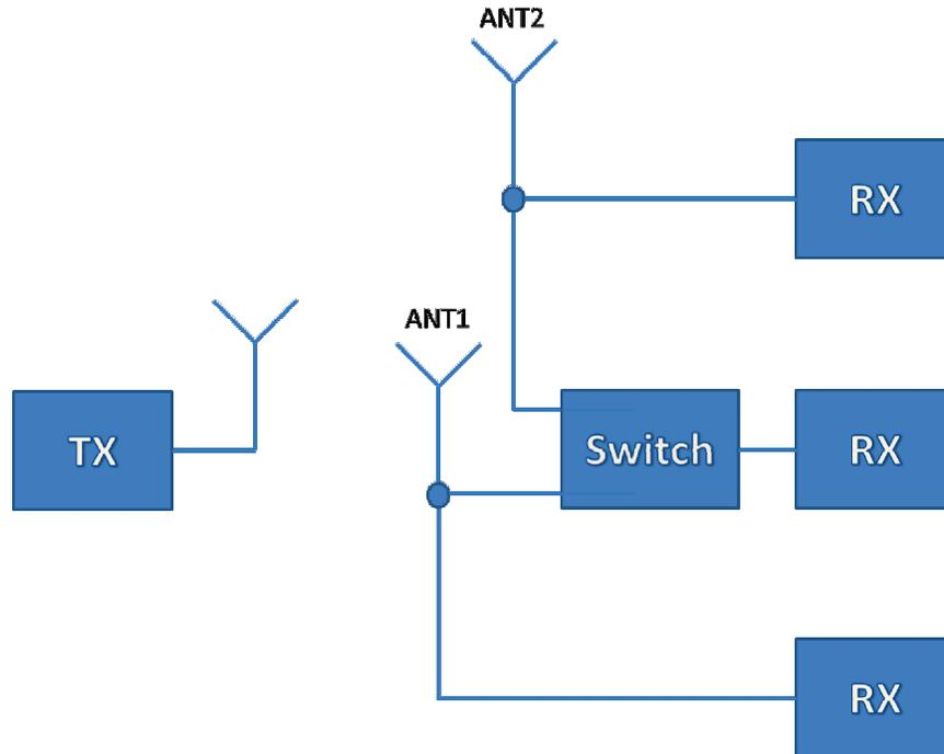
Figure 2. Block Diagram of Antenna Diversity Test Setup
