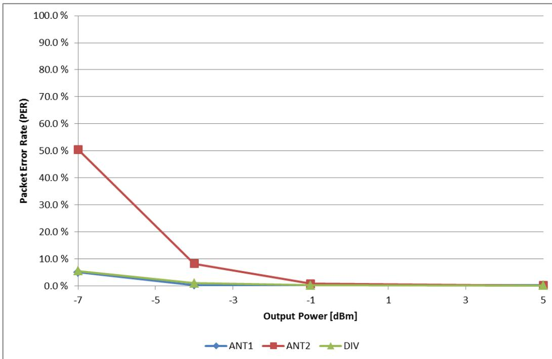
Figure 5. Packet Error Rate vs Output Power. Test Setup 4
