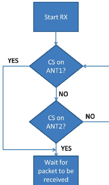
**Figure 1. Simplified Flowchart for CC1200-Based Antenna Diversity**
