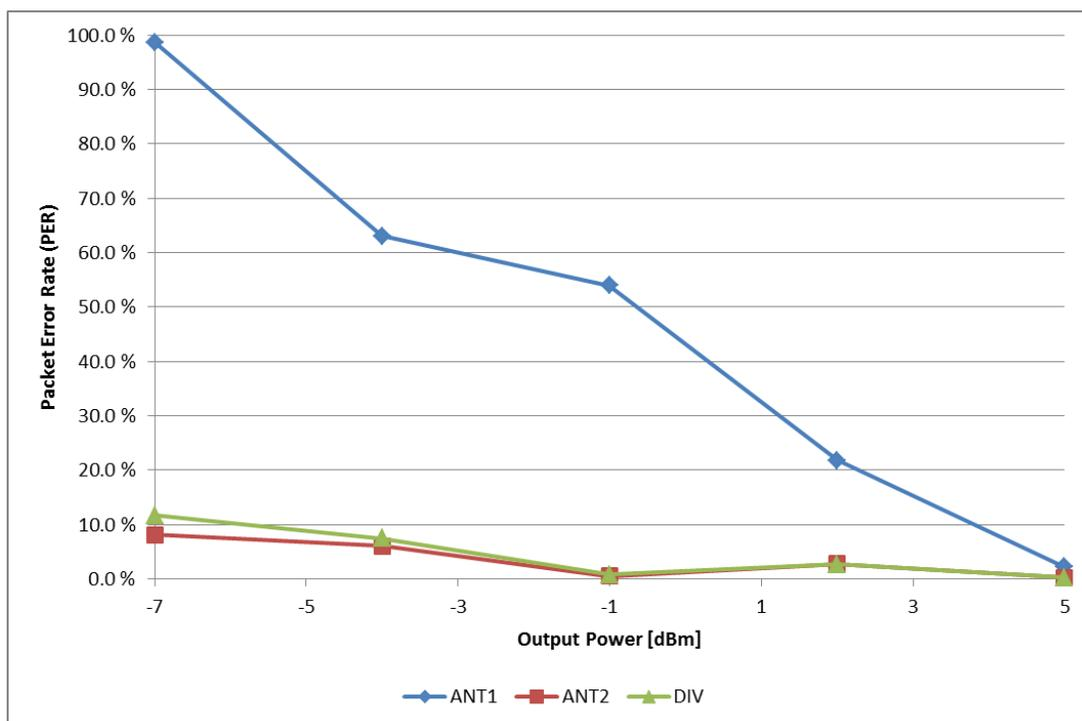
**Figure 4. Packet Error Rate vs Output Power. Test Setup 3**
