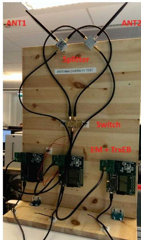
**Figure 3. Antenna Diversity Test Board**
