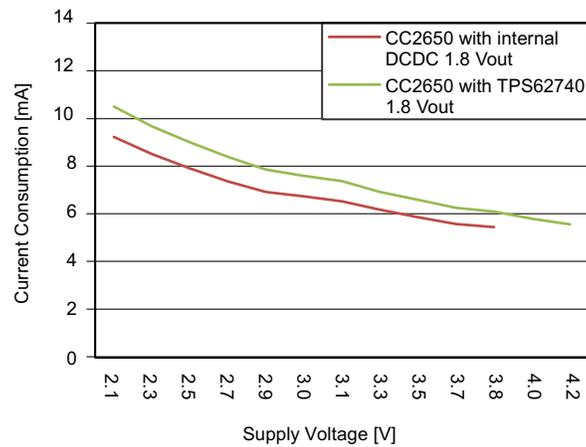
Figure 3. Power Consumption in TX, 0 dBm Setting
