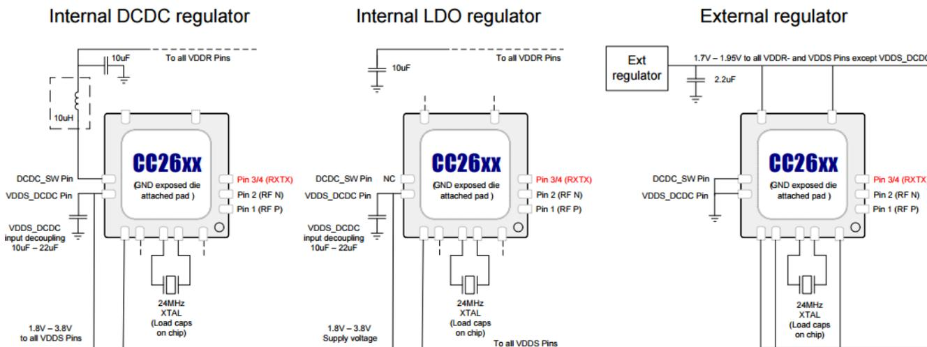
Figure 1. Simplified CC26xx Family Power Supply Configuration
