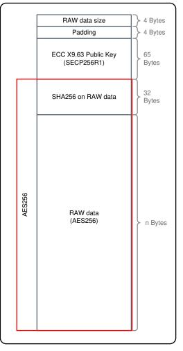
Figure 5-2. Secure Content Delivery – File Format
