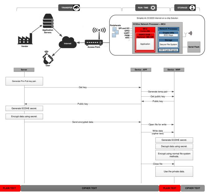
Figure 5-1. Secure Content Delivery – Process Description
