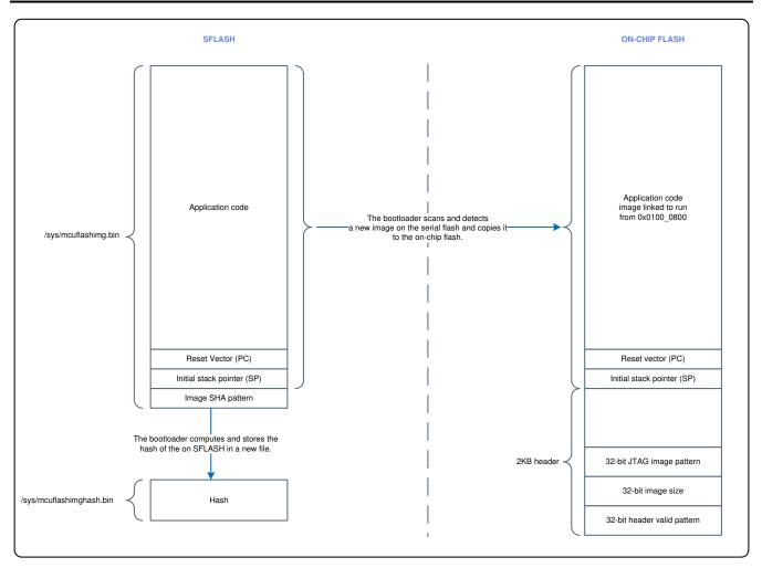
Figure 7-1. On-Chip Flash Programming and Update
