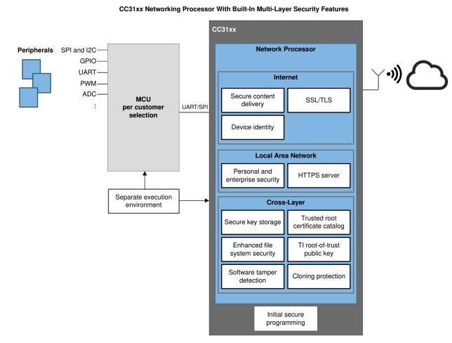
Figure 1-4. CC3120/CC3130/CC3135 Device Security Features
