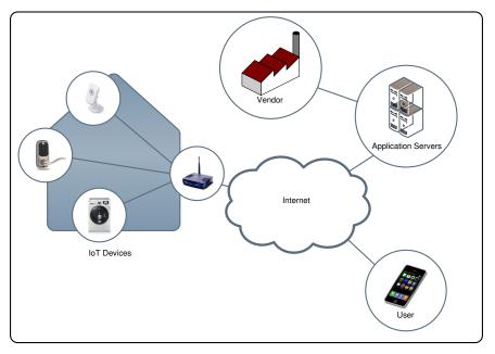
Figure 1-1. Common Exposure Points of IoT Devices
