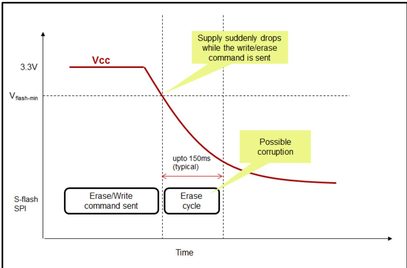
**Figure 1. Sudden Power Off During Flash Erase**
