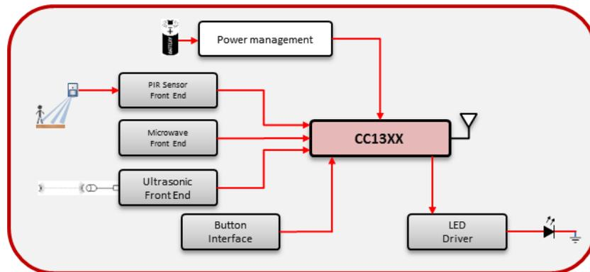
**Figure 3-1. Motion Detection System Block Diagram**
