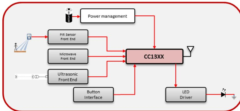
**Figure 3-1. Motion Detection System Block Diagram**
