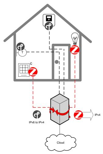
Figure 1. Thread and Zigbee<sup>®</sup> Cloud Access Flow
