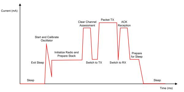
Figure 3. Typical Power Envelope in Thread and Zigbee<sup>®</sup>
