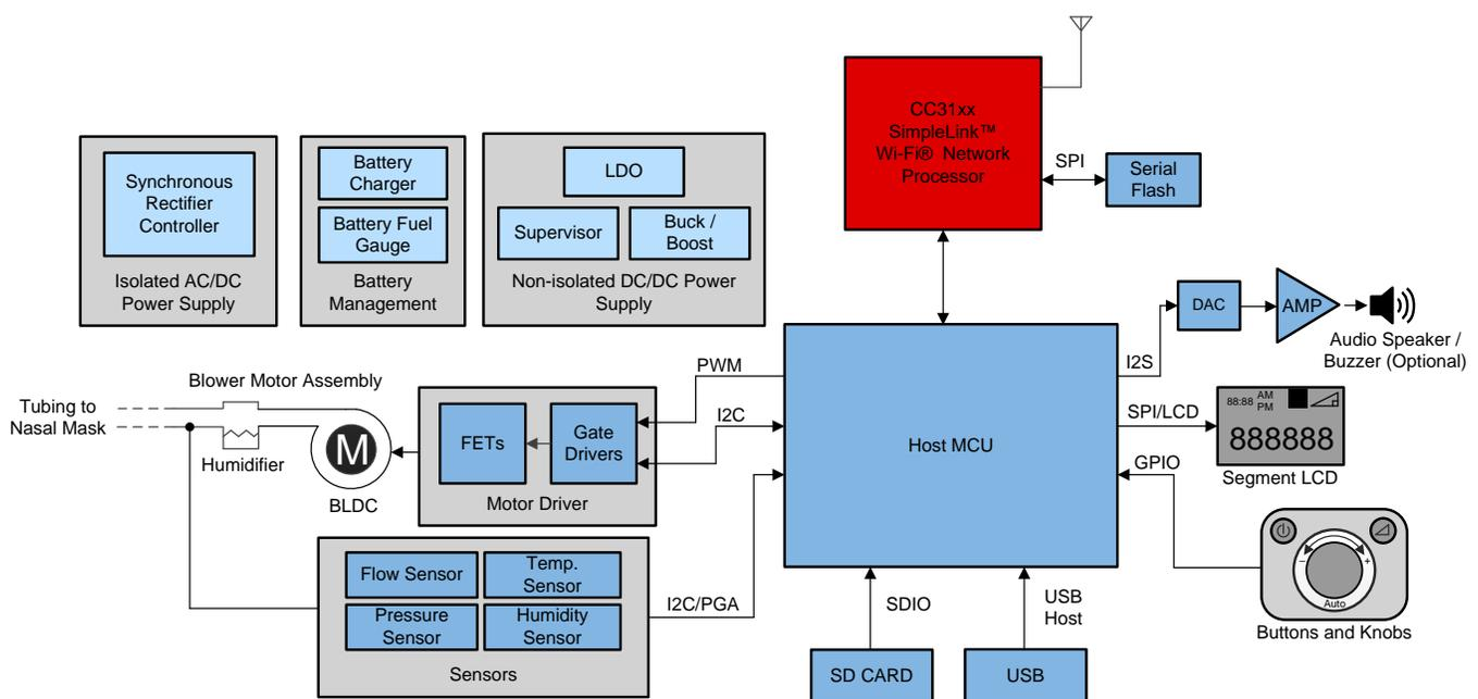
**Figure 3. CPAP Machine Block Diagram Using the CC3120 SimpleLink Wi-Fi NWP**
