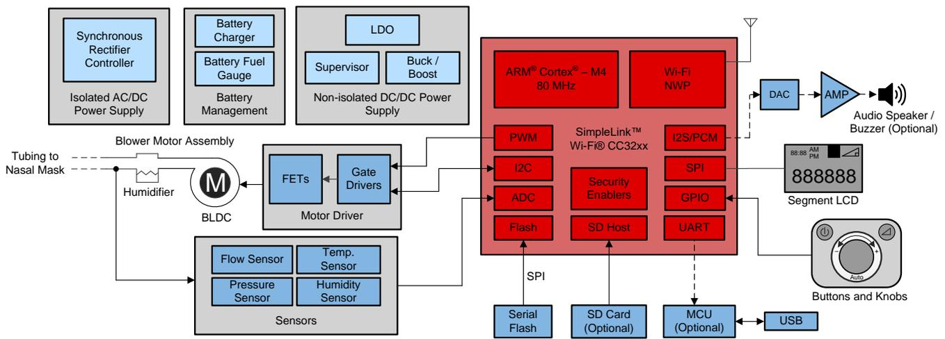
**Figure 2. CPAP Machine Block Diagram Using the CC3220 SimpleLink Wi-Fi Wireless MCU**
