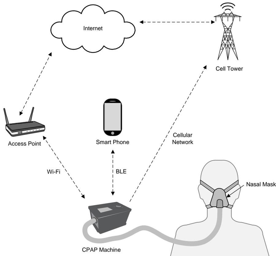
**Figure 1. Connected CPAP Use Cases**
