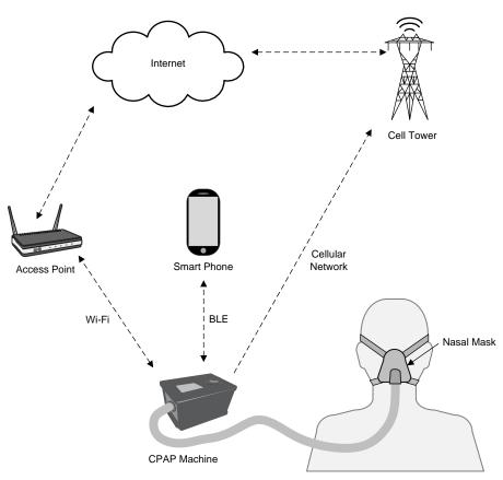
Figure 1. Connected CPAP Use Cases
