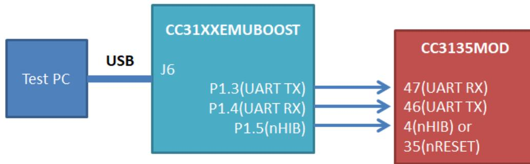
**Figure 4. Programming Through USB**
