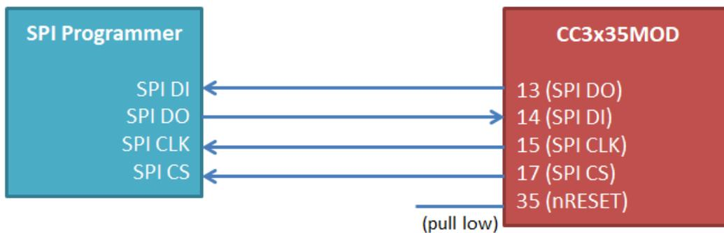
Figure 5. Programming Through SPI
